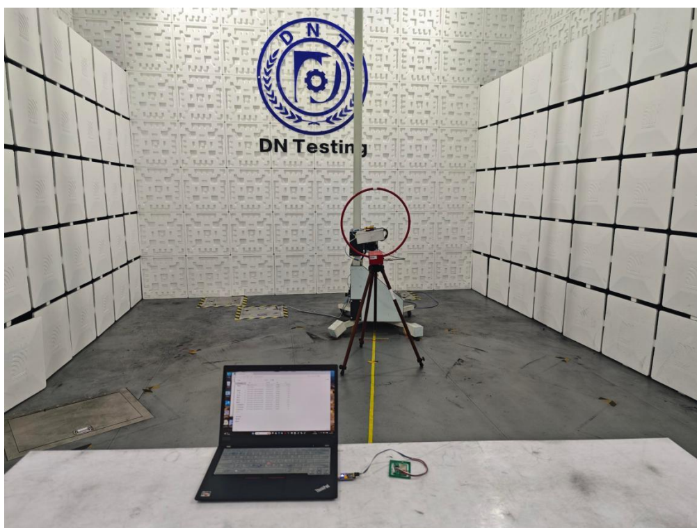
Radiated Emission Test View(9KHz-30MHz)
