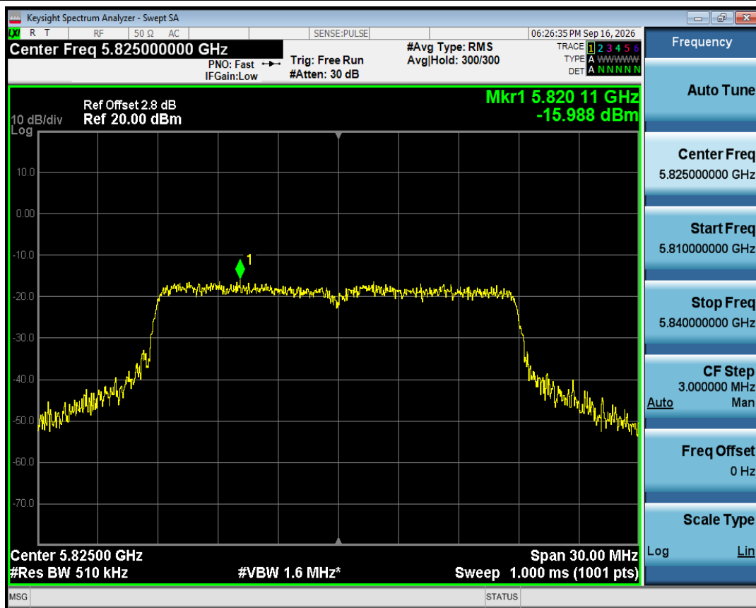
PSD NVNT n20 5825MHz Ant1
