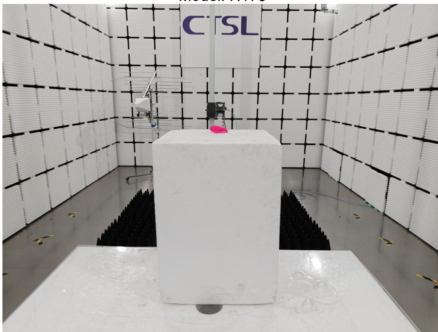
Photo 2 Test Setup Photos of Radiated Emission Test (Above 1GHz) Model: H179
