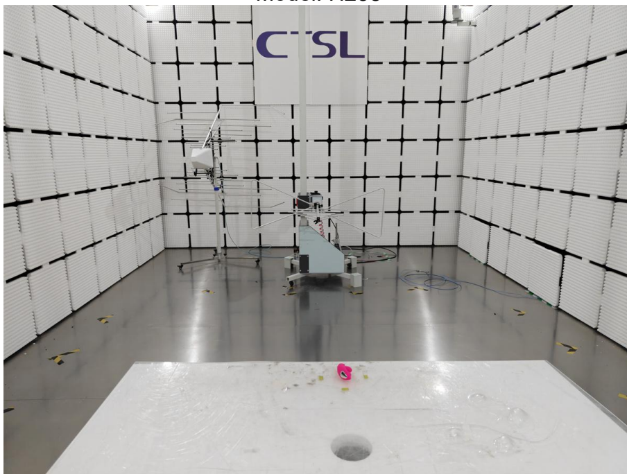
Photo 8 Test Setup Photos of Radiated Emission Test (30-1000MHz)
