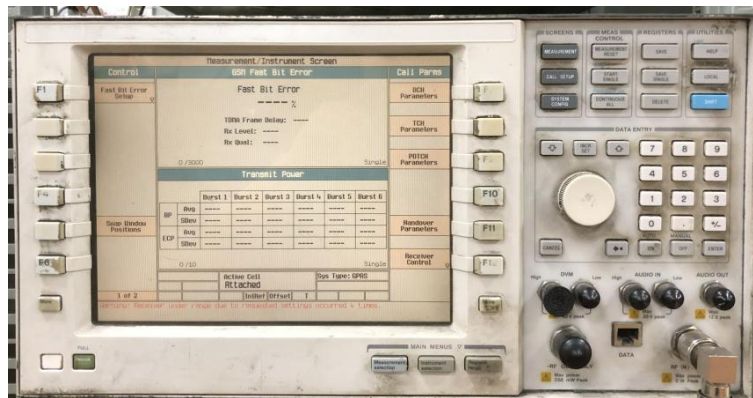
Agilent 8960 (2G/3G Test Equipment)
