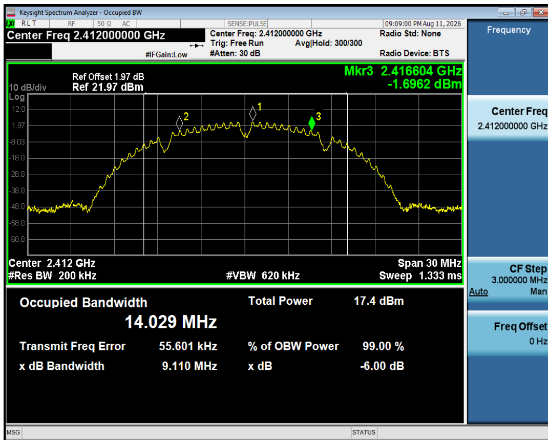
-6dB Bandwidth NVNT b 2412MHz Ant1
