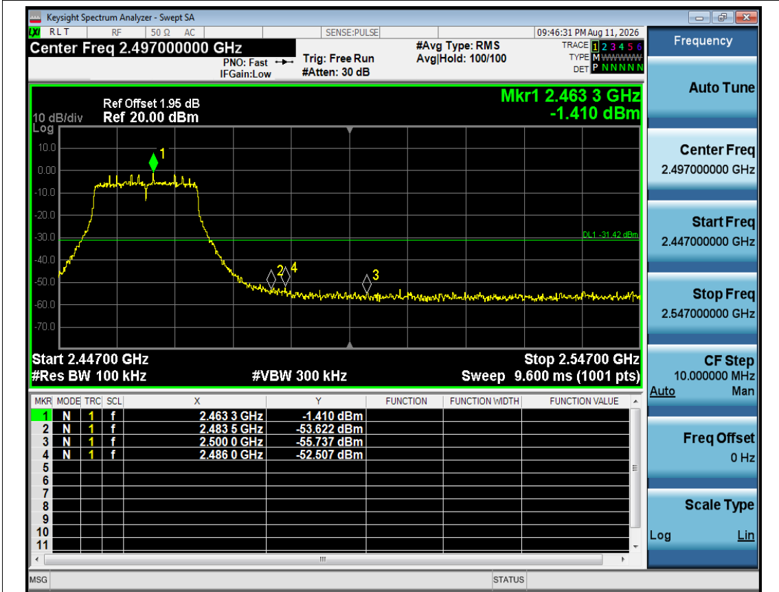
Band Edge NVNT n20 2462MHz Ant1 Emission
