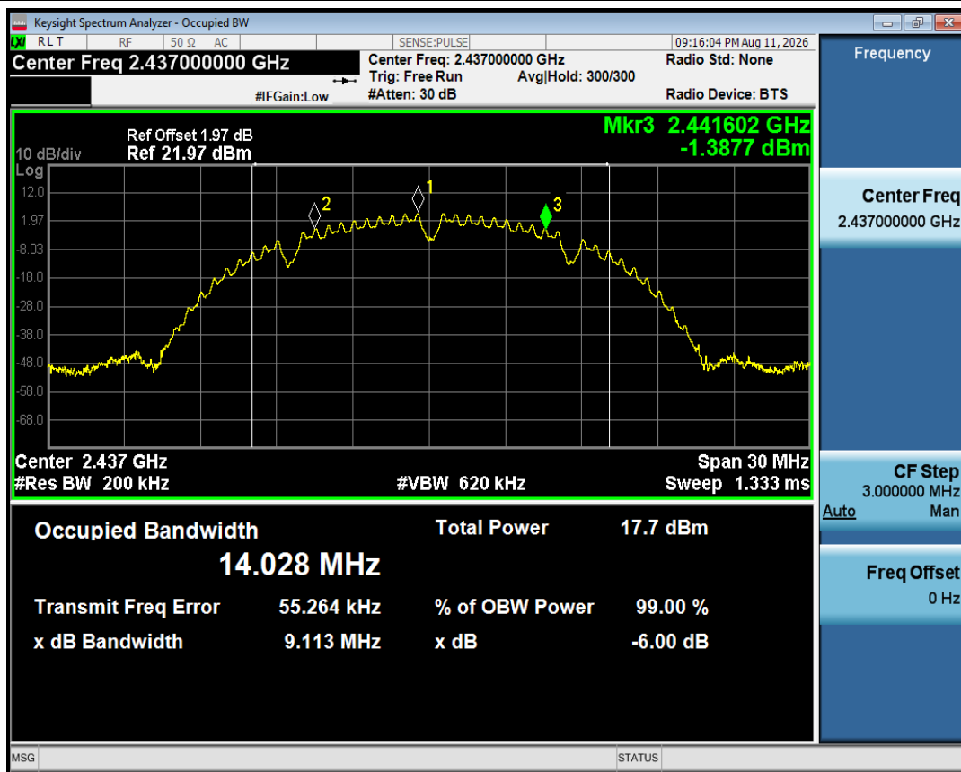
-6dB Bandwidth NVNT b 2437MHz Ant1
