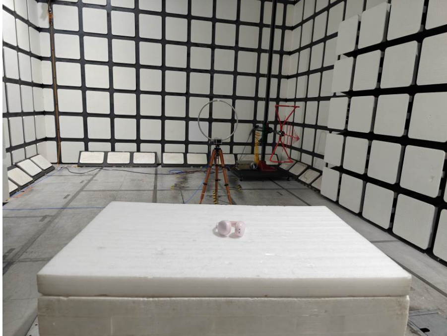
Radiated Emissions View (Below 30MHz)
