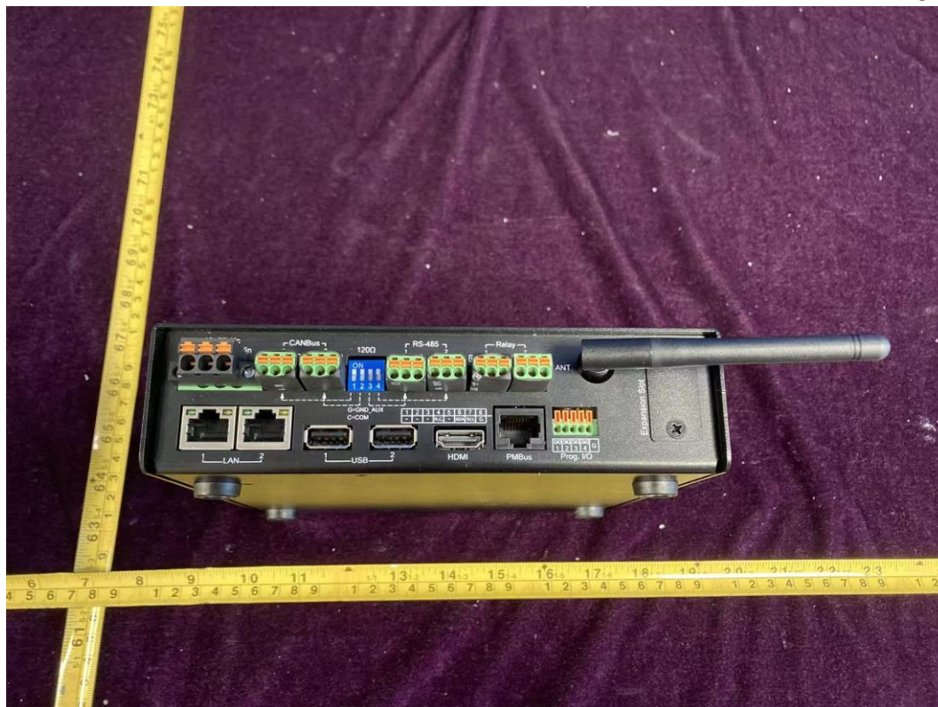
FIGURE 6 MULTI-INDUSTRY GENERAL PURPOSE SMART CONTROLLER (M/N: CMU3) OUT-6
