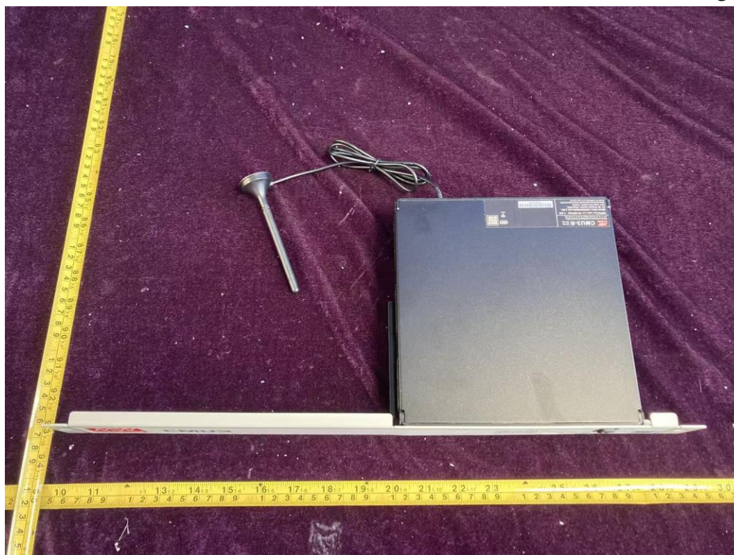
FIGURE 7 MULTI-INDUSTRY GENERAL PURPOSE SMART CONTROLLER (M/N: CMU3-R) OUT-1
