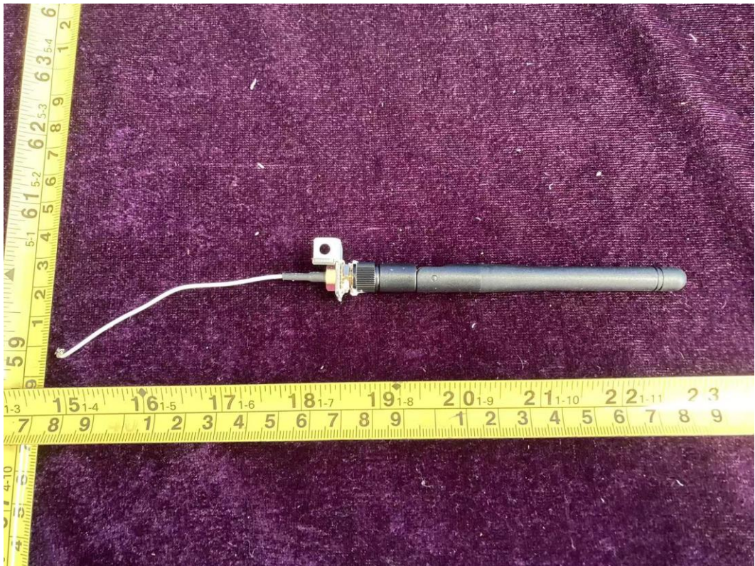
FIGURE 36 MULTI-INDUSTRY GENERAL PURPOSE SMART CONTROLLER (M/N: CMU3) ANTENNA
