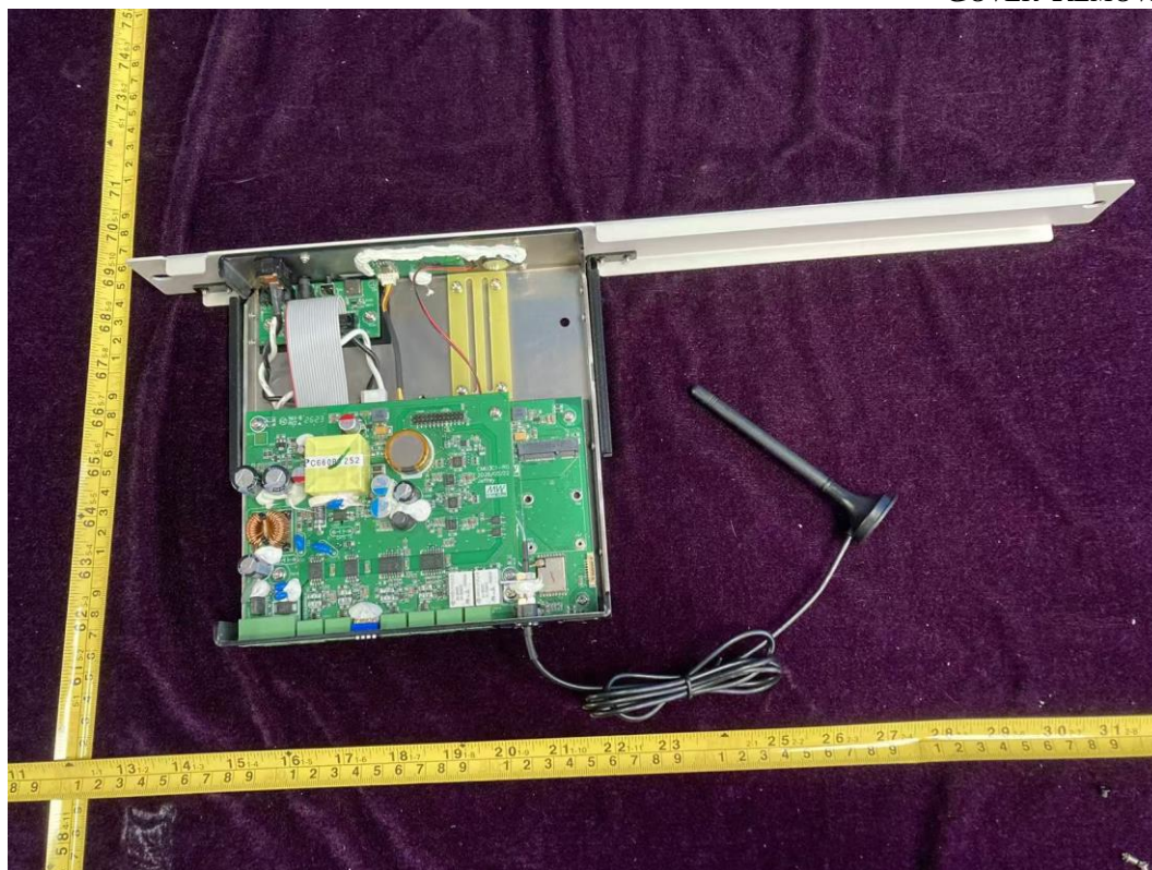
FIGURE 14 MULTI-INDUSTRY GENERAL PURPOSE SMART CONTROLLER (M/N: CMU3-R) COVER REMOVED 2
