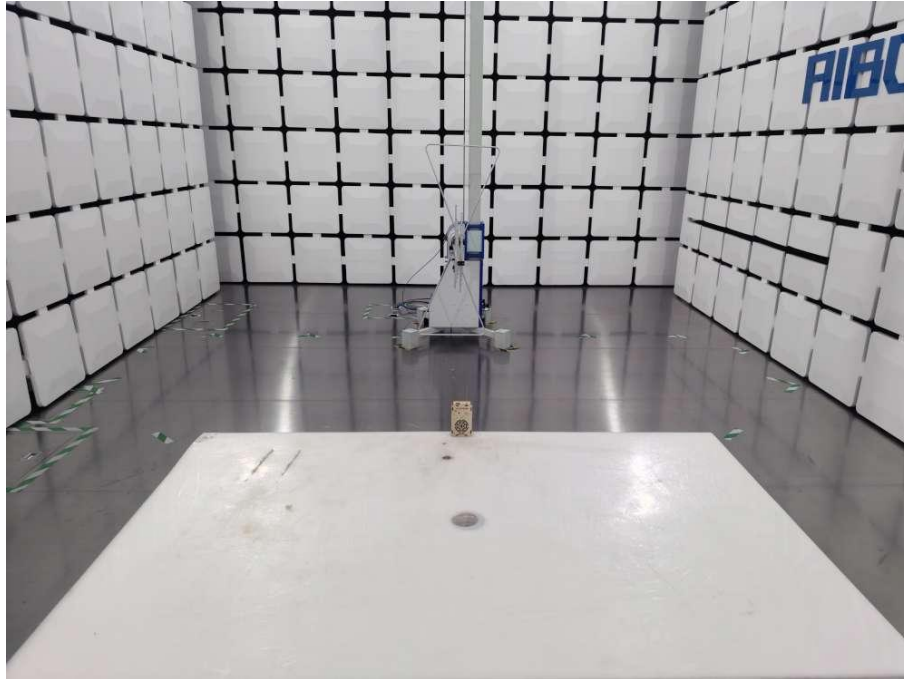
Radiated Emission Test View Below 1GHz
