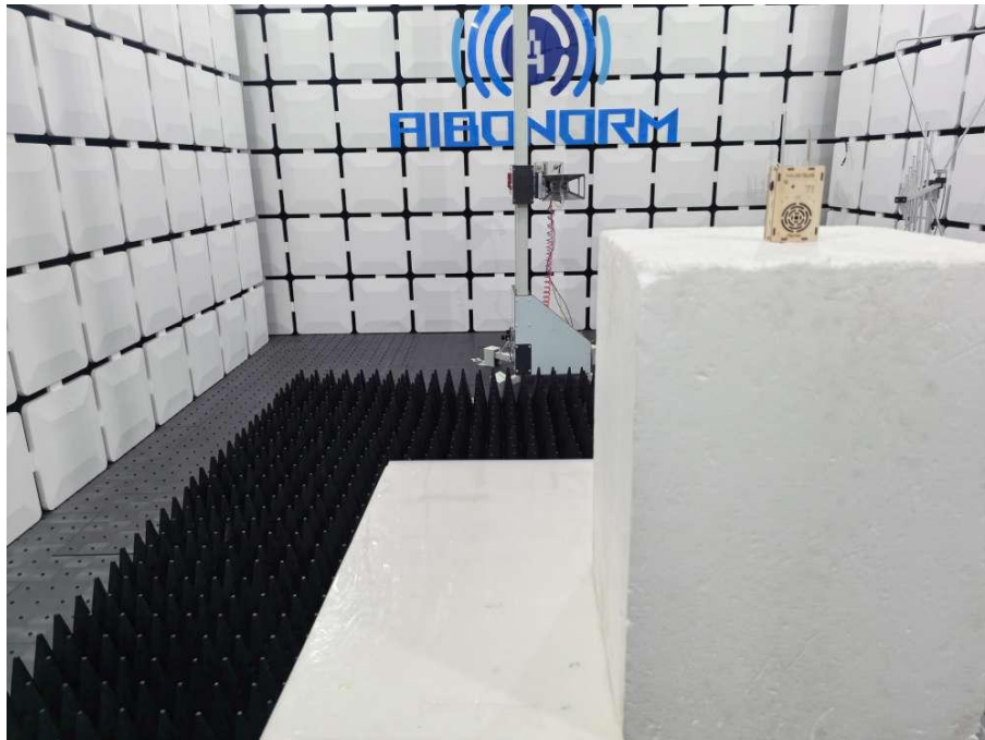
Radiated Emission Test View Above 1GHz
