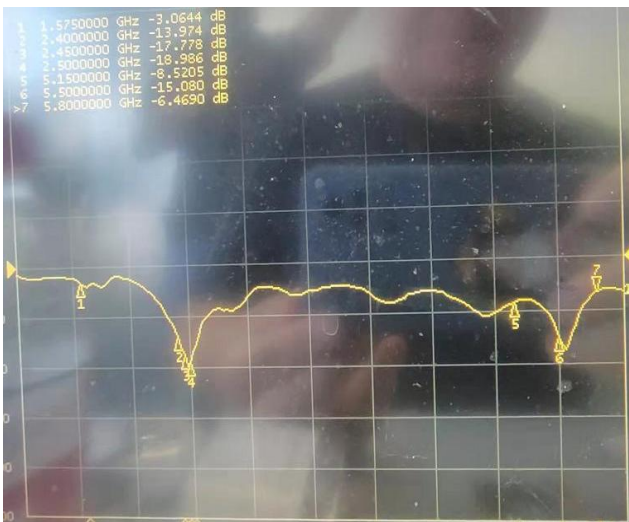
2.4G WIFI Standing wave return loss graph
