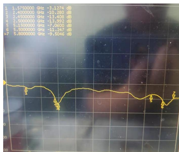
5.8G WIFI Standing wave return loss graph
