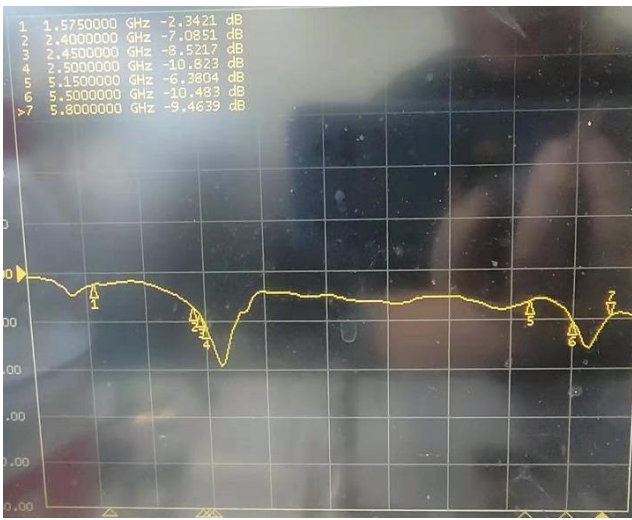
2.4G BT Standing wave return loss graph
