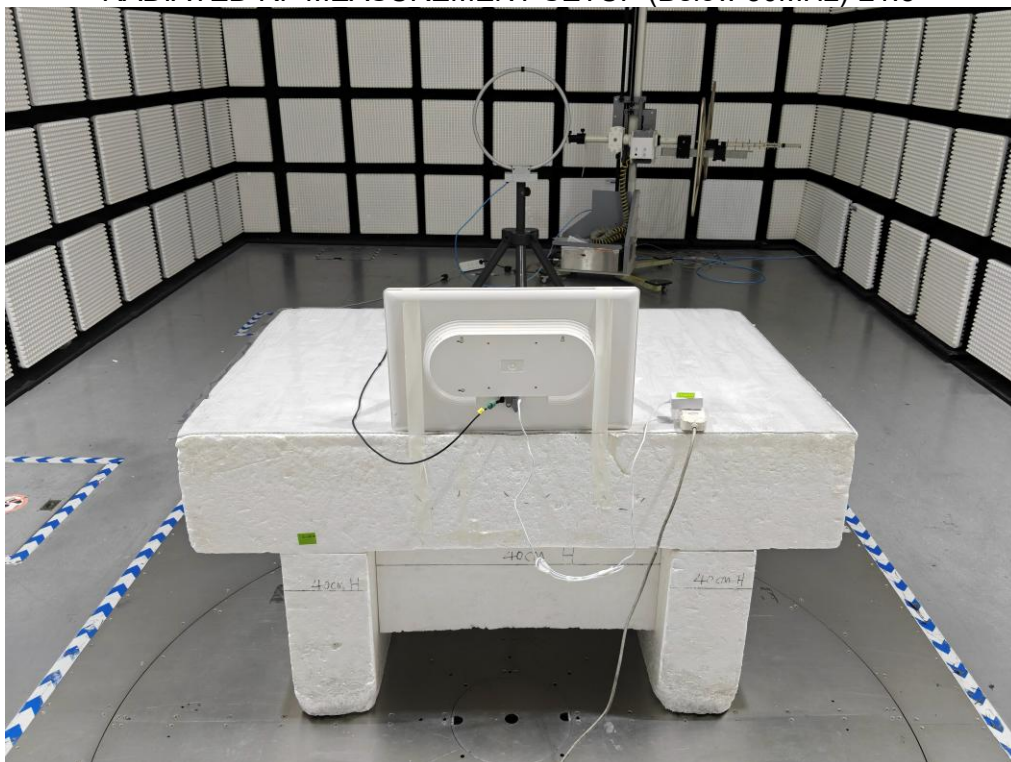
RADIATED RF MEASUREMENT SETUP (Below 30MHz)-21.5'
