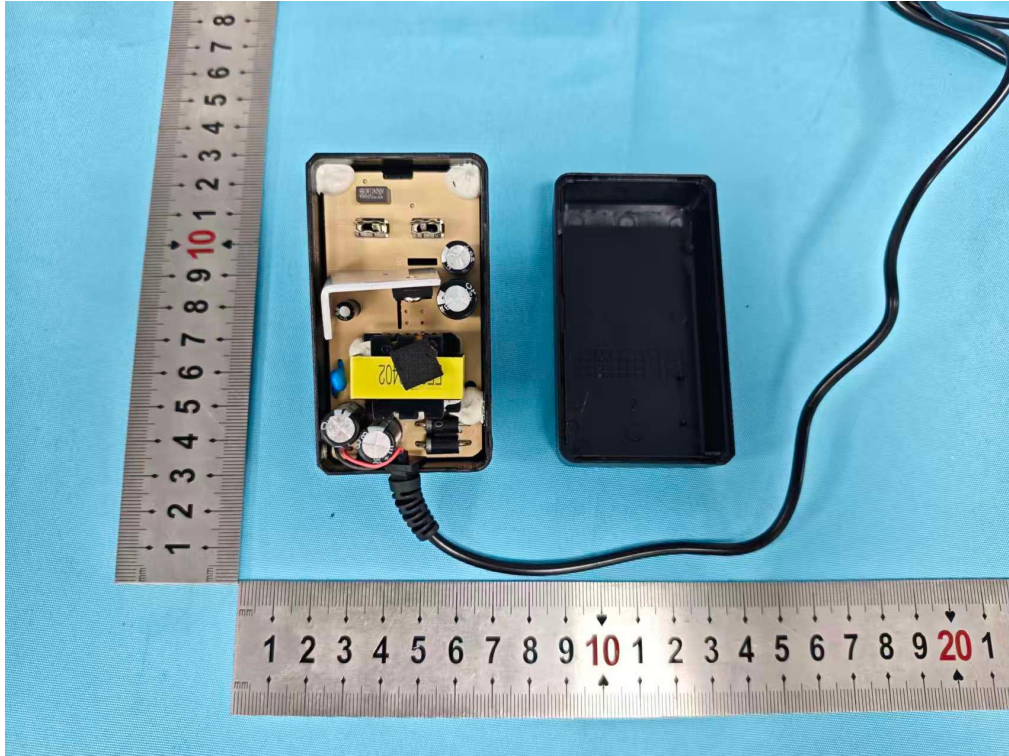
Photo 5 Internal photos of EUT
