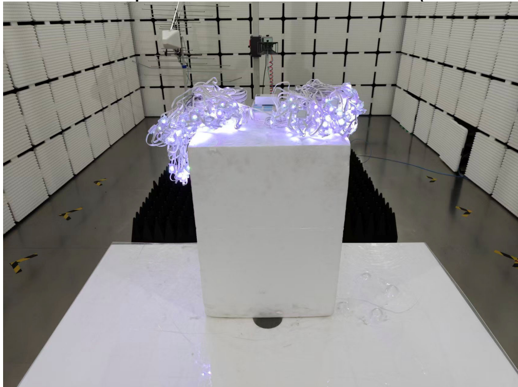
Photo 2 Test Setup Photos of Radiated Emission Test (Above 1GHz)
