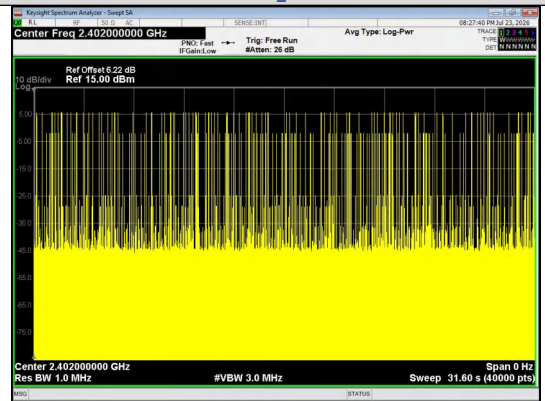
Number of Pulses in 31.6 seconds \pi/4 DQPSK_2-DH5
