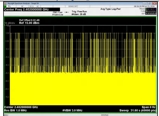
Number of Pulses in 31.6 seconds 8DPSK_3-DH5
