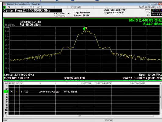
Out Of Band Emission \pi/4 DQPSK_2-DH5_Channel 39
