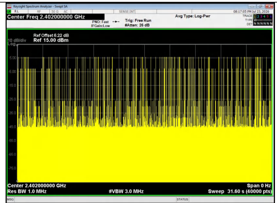
Number of Pulses in 31.6 seconds GFSK_DH5
