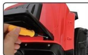
4.Align the front windshield buckle with the body groove and insert it into the screw holes on both sides,and then fix and lock it with screws.
