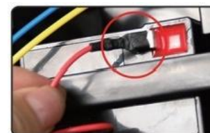
2.Connect the red end corresponding to the red line to the battery cable
