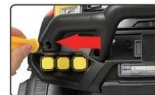
6. Align the front bumper with the four recessed holes in the front as shown in the picture and insert them,then tighten and fix them one by one with screws.
