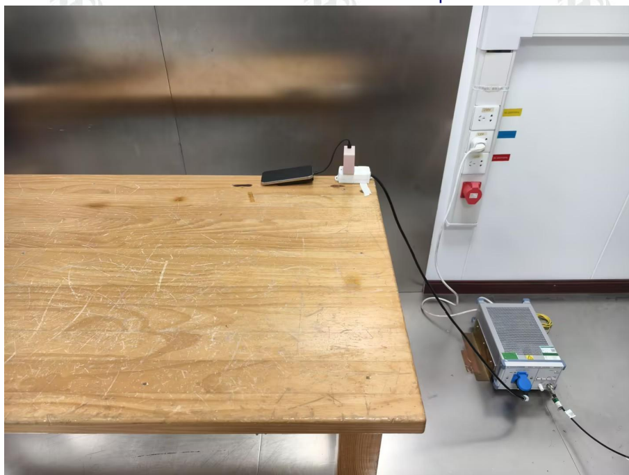
Conducted Emission Test Setup
