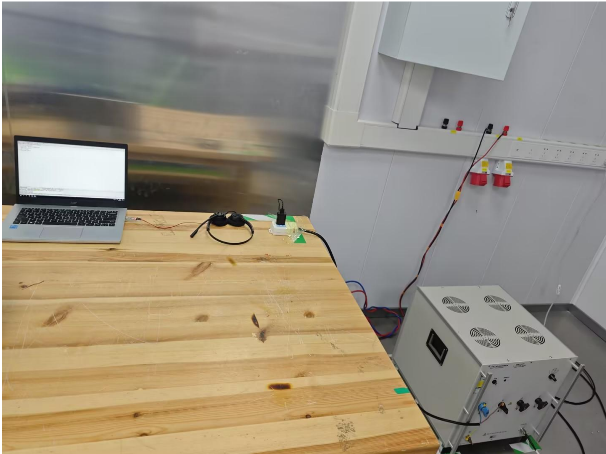
AC Power Line Conducted Emissions Test View
