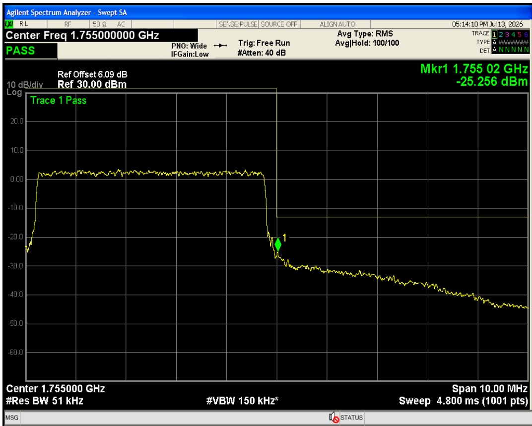
Band4 QAM16 BW=10MHz Channel=20000 RB Size=50 Position=#0
