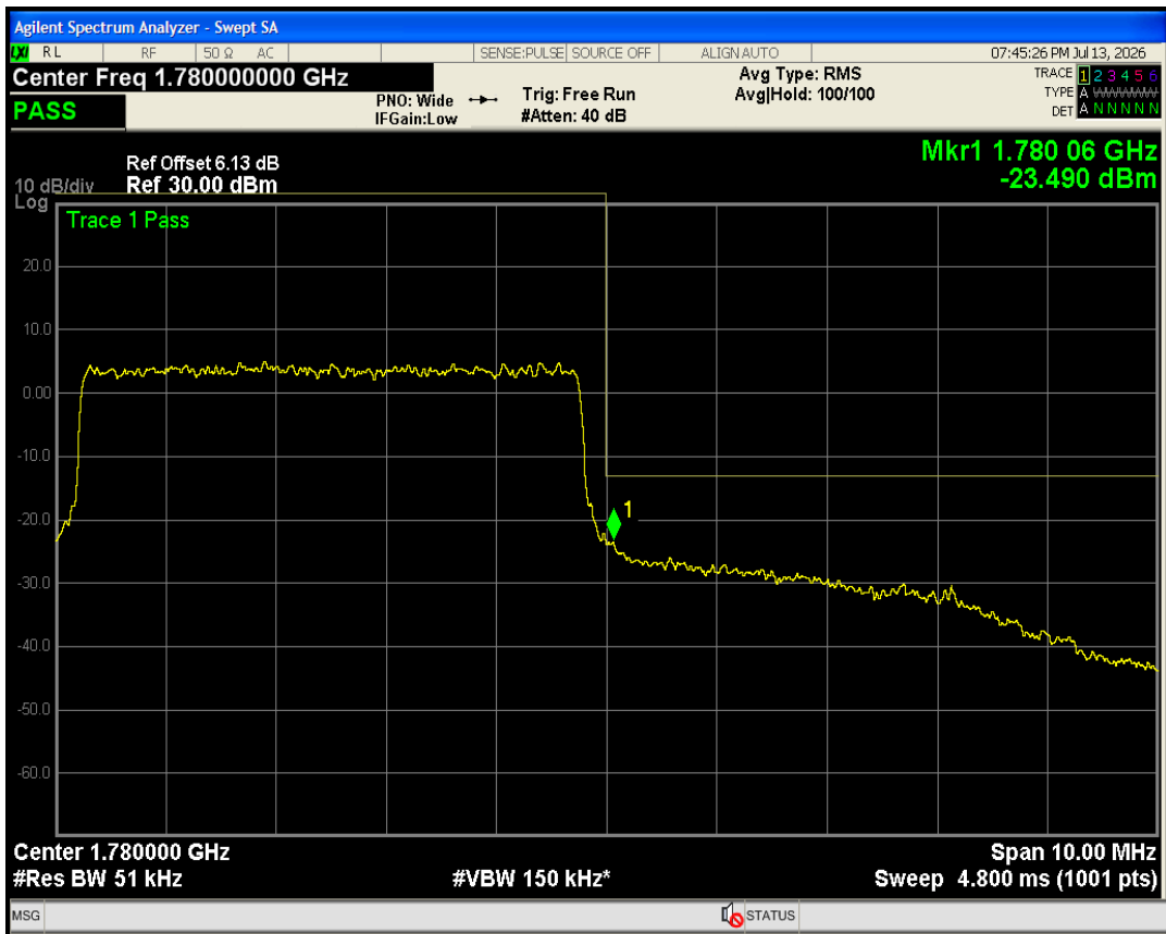
Band66 QAM16 BW=5MHz Channel=132647 RB Size=25 Position=#0
