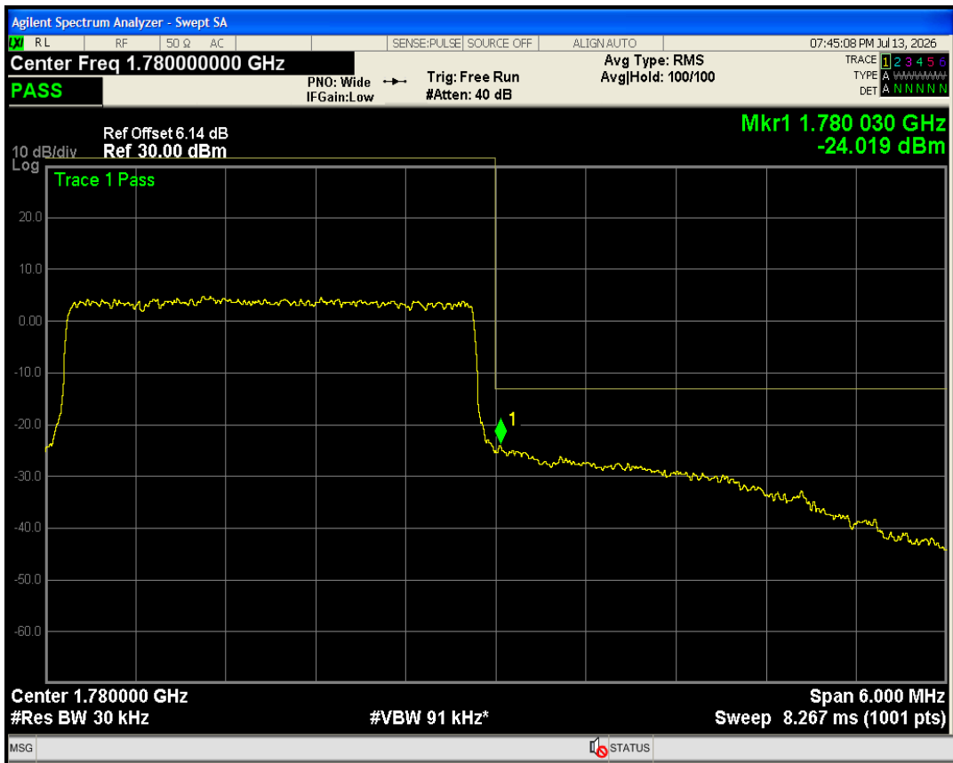
Band66 QAM16 BW=3MHz Channel=132657 RB Size=15 Position=#0
