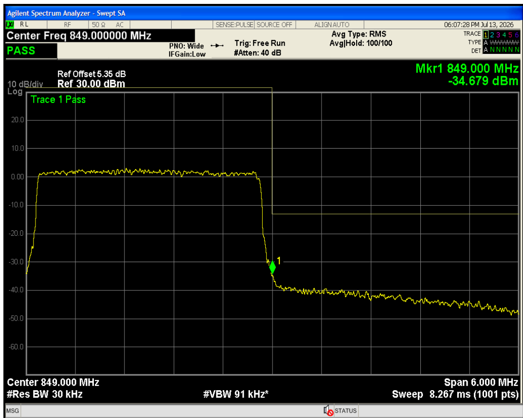
Band5 QPSK BW=5MHz Channel=20425 RB Size=25 Position=#0
