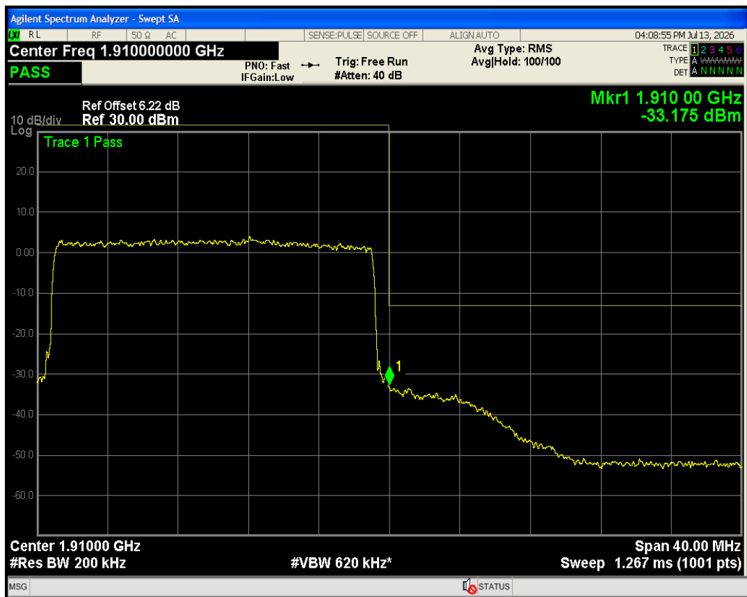
Band4 QAM16 BW=1.4MHz Channel=19957 RB Size=6 Position=#0
