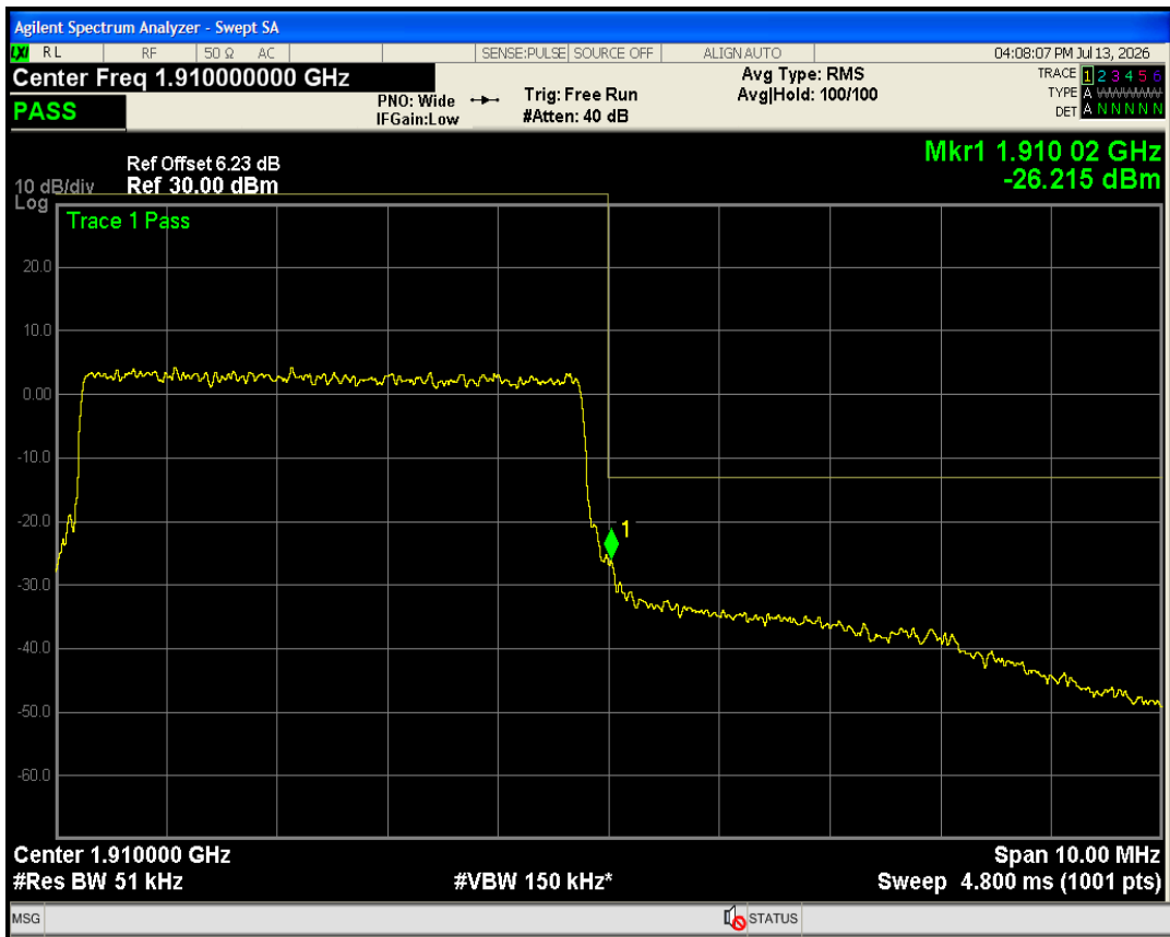
Band2 QAM16 BW=10MHz Channel=18650 RB Size=50 Position=#0
