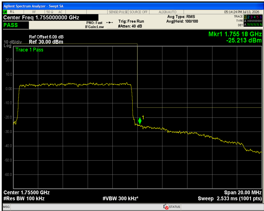
Band4 QAM16 BW=10MHz Channel=20350 RB Size=50 Position=#0
