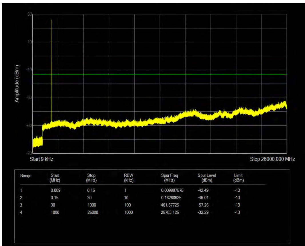
Band2 QPSK BW=3MHz Channel=18615 RB Size=15 Position=#0
