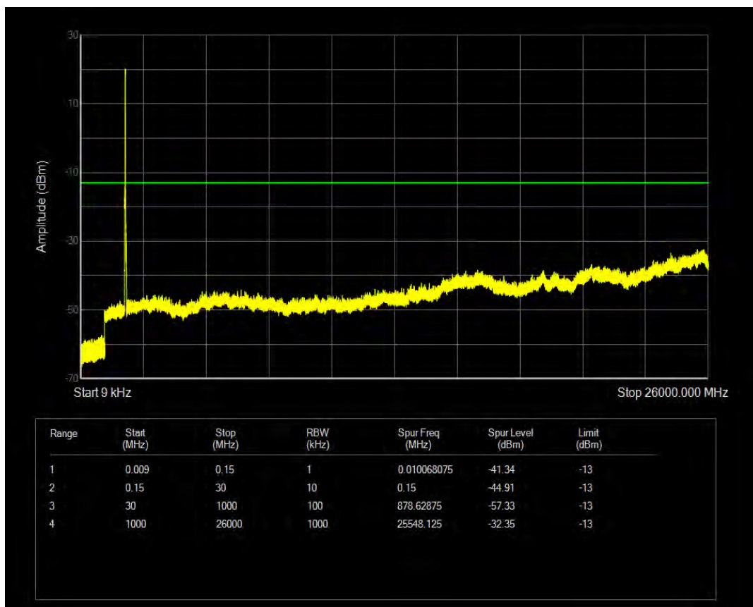
Band2 QAM16 BW=10MHz Channel=19150 RB Size=50 Position=#0
