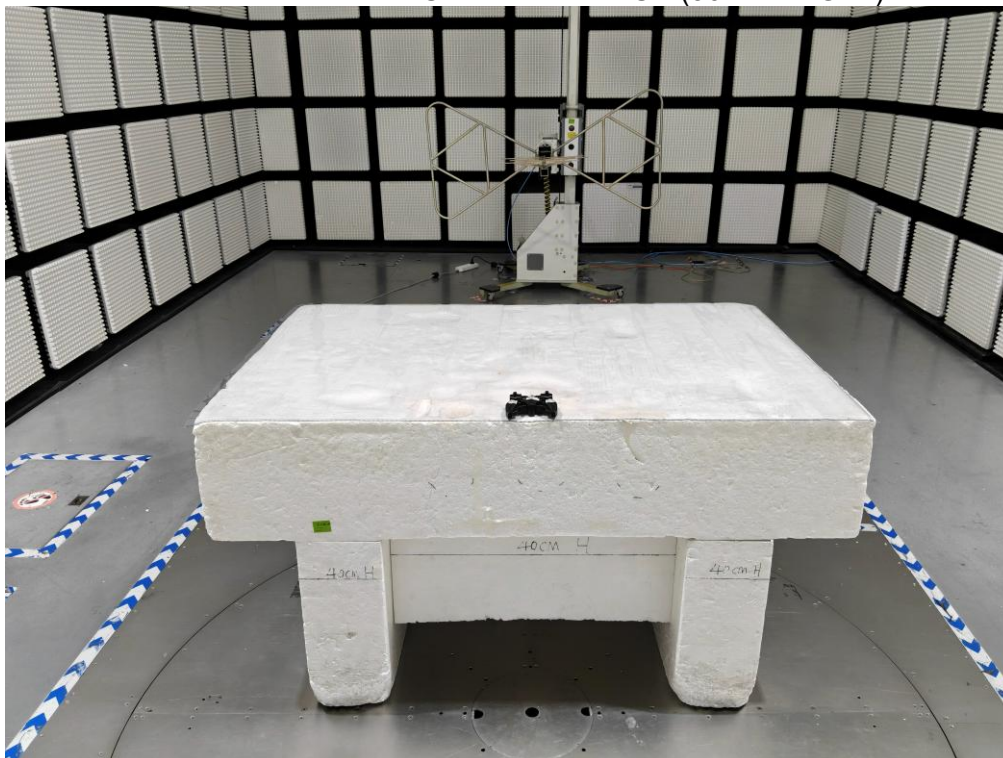
RADIATED RF MEASUREMENT SETUP (30MHz~1GHz)
