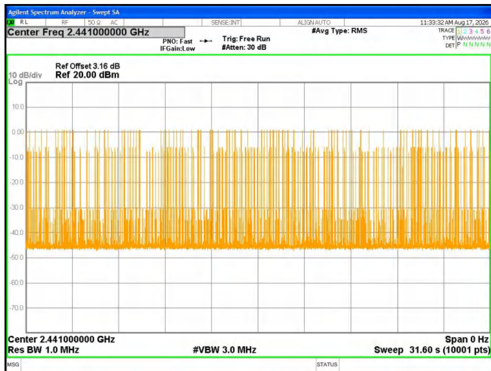
Dwell NVNT 1-DH5 2441MHz Ant1 Accumulated
