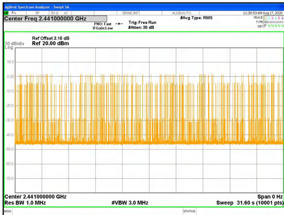
Dwell NVNT 2-DH5 2441MHz Ant1 Accumulated
