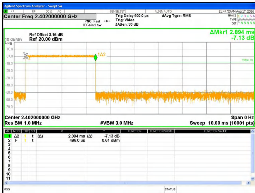
Dwell NVNT 3-DH5 2402MHz Ant1 One Burst
