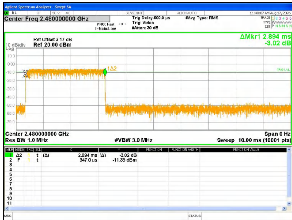
Dwell NVNT 3-DH5 2480MHz Ant1 One Burst
