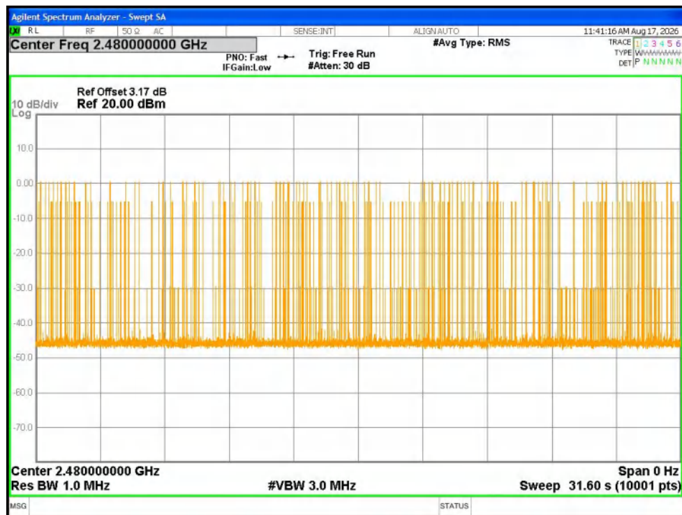
Dwell NVNT 2-DH5 2480MHz Ant1 Accumulated
