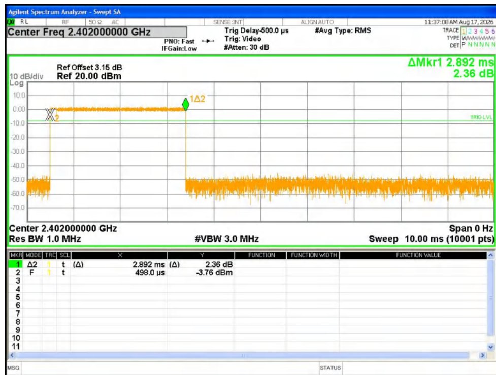
Dwell NVNT 2-DH5 2402MHz Ant1 One Burst
