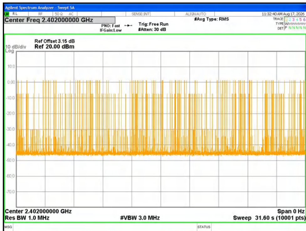
Dwell NVNT 1-DH5 2402MHz Ant1 Accumulated
