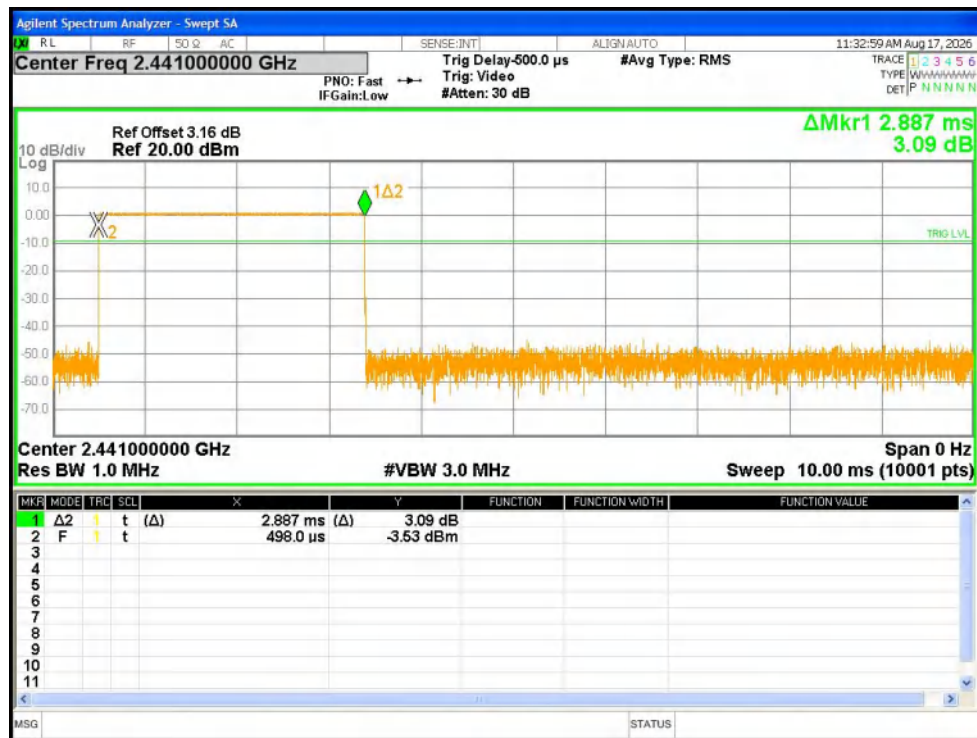
Dwell NVNT 1-DH5 2441MHz Ant1 One Burst
