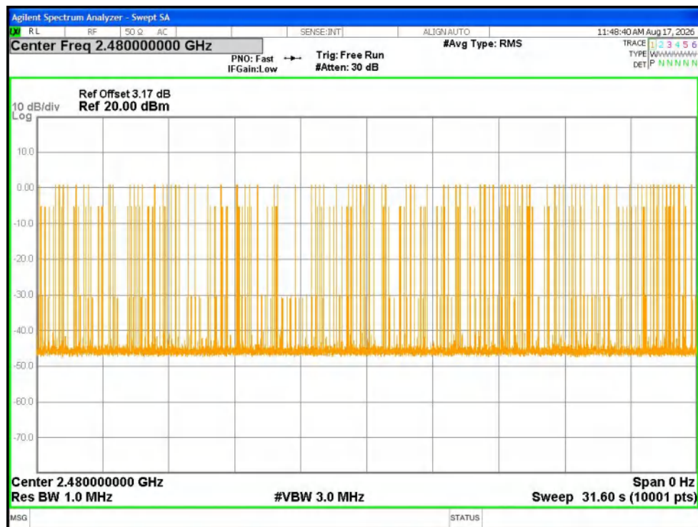
Dwell NVNT 3-DH5 2480MHz Ant1 Accumulated
