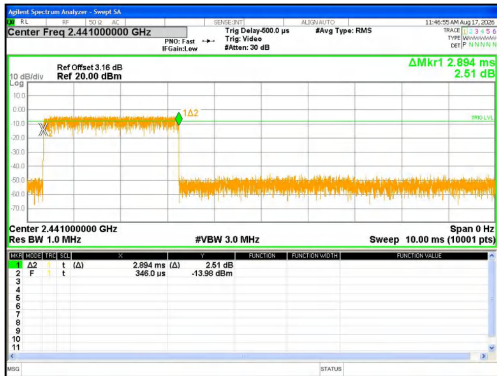
Dwell NVNT 3-DH5 2441MHz Ant1 One Burst
