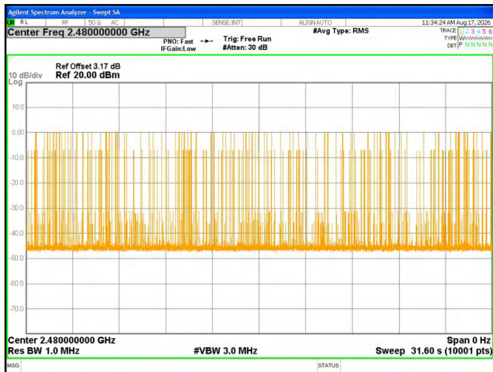
Dwell NVNT 1-DH5 2480MHz Ant1 Accumulated
