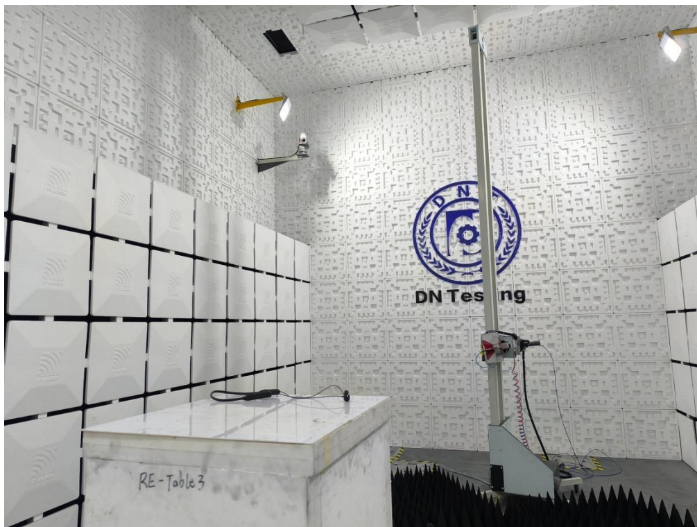
Radiated Emission Test View|(Above 1G)
