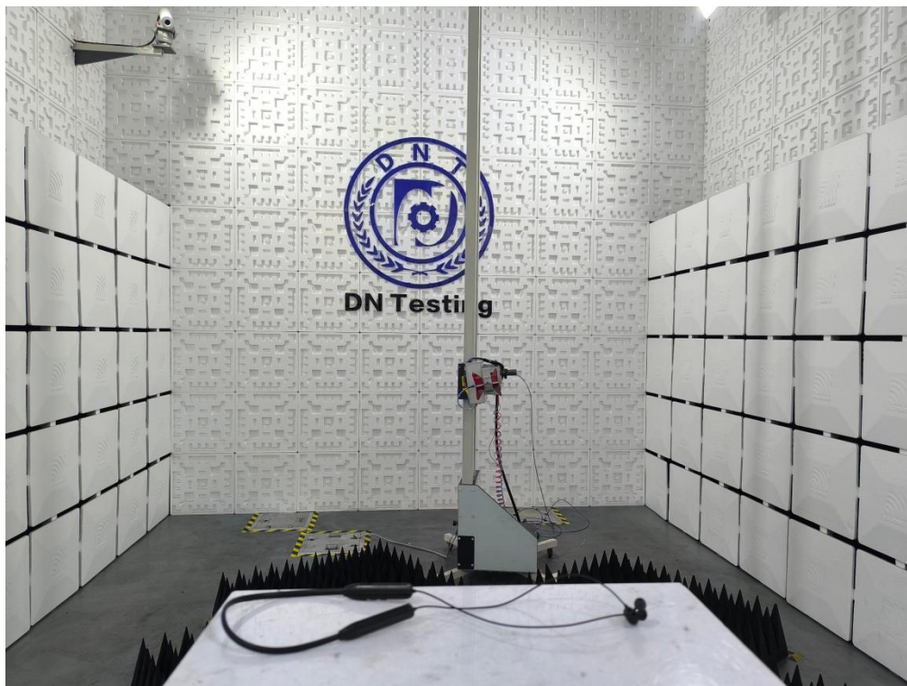
Radiated Emission Test View|(Above 1G)
