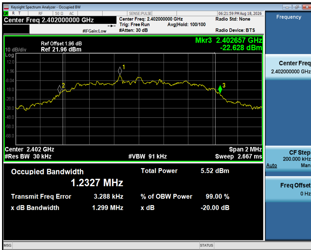
-20dB Bandwidth NVNT 3-DH5 2402MHz Ant1
