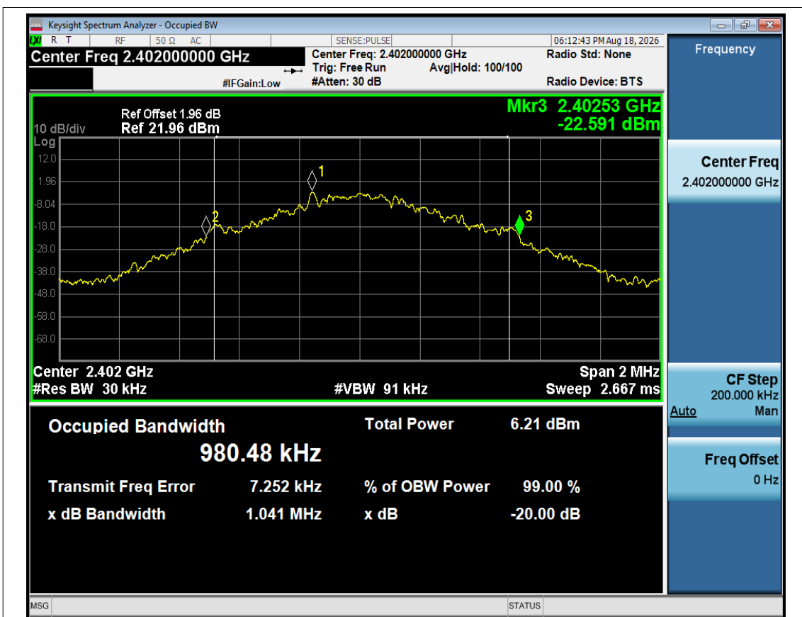
-20dB Bandwidth NVNT 1-DH5 2402MHz Ant1
