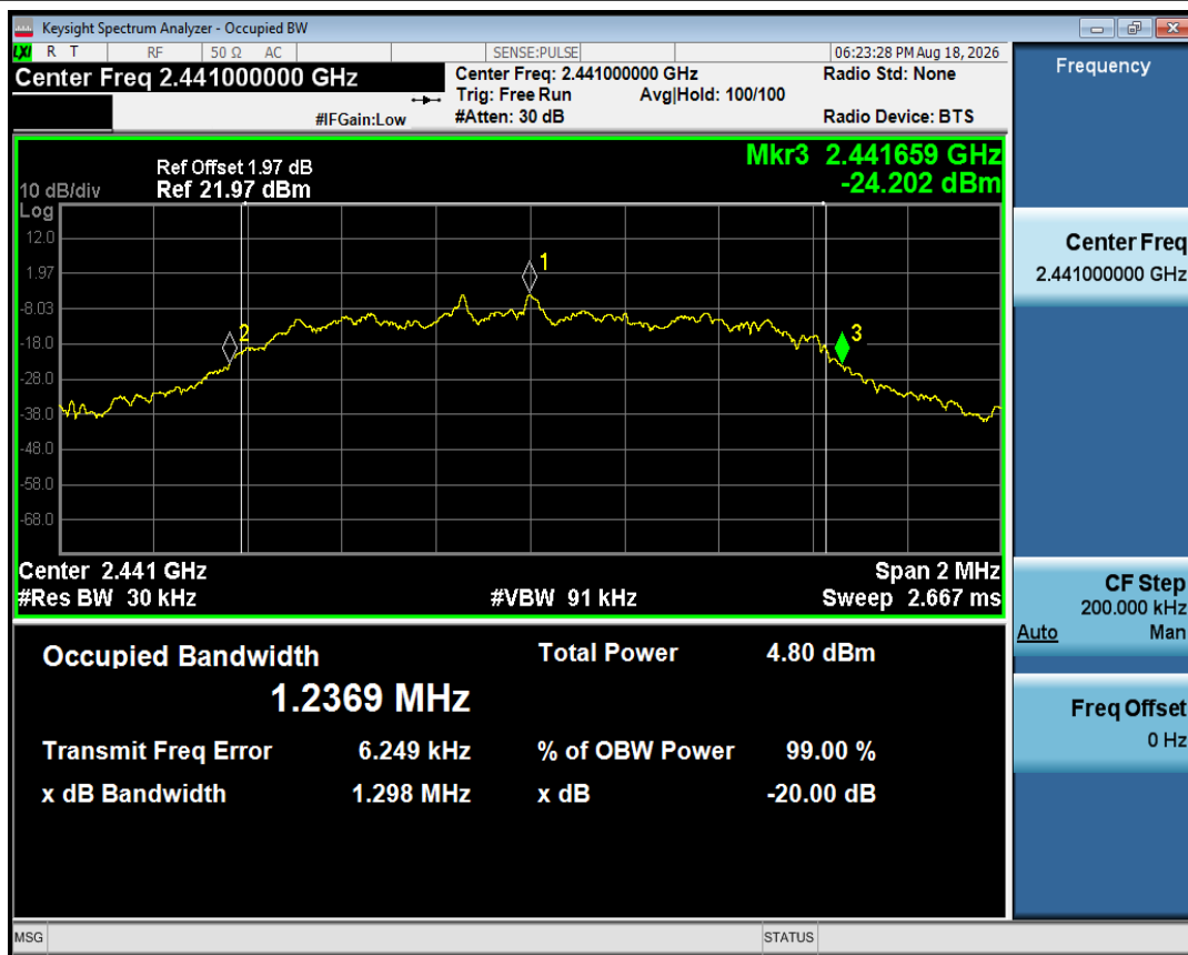
-20dB Bandwidth NVNT 3-DH5 2441MHz Ant1
