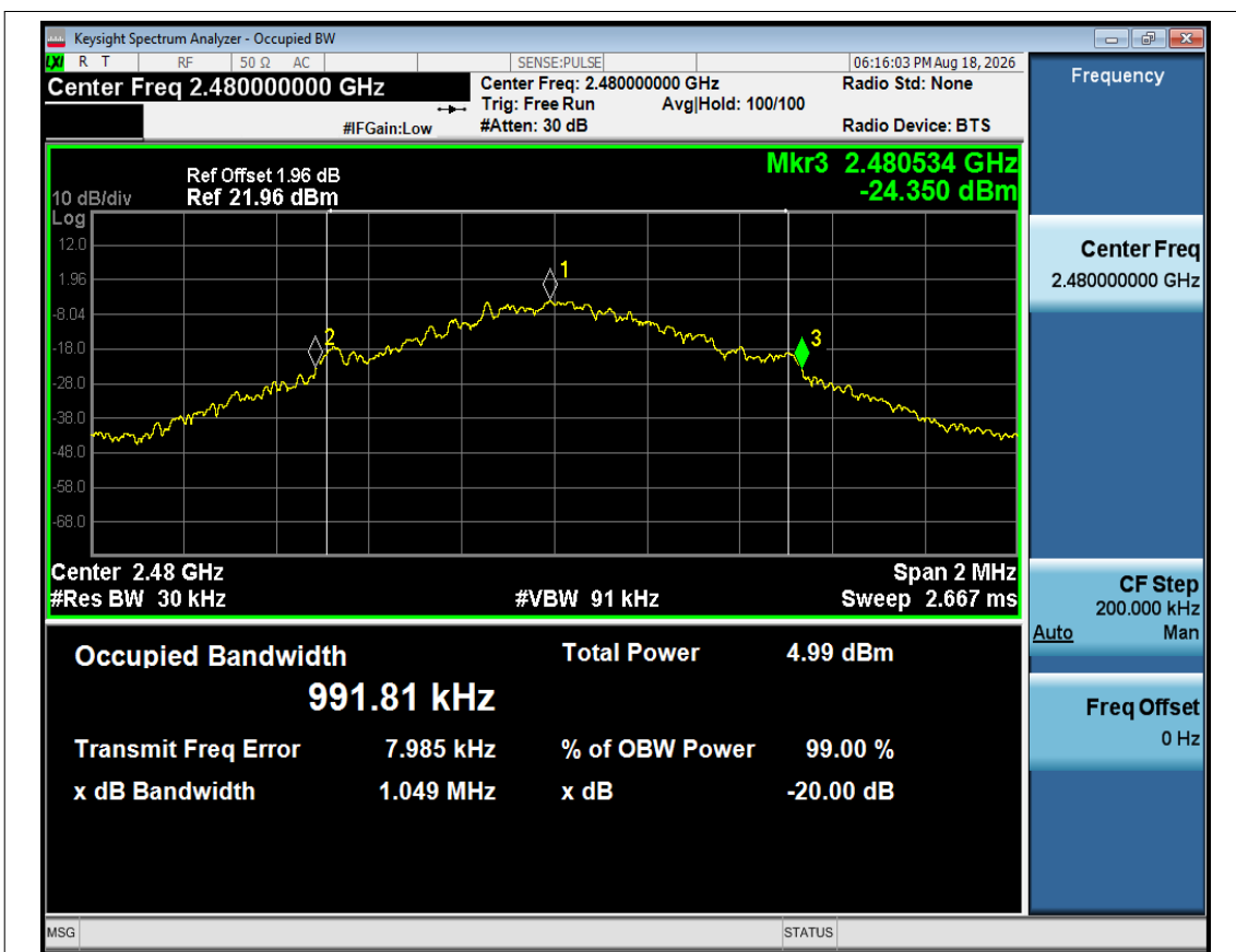
-20dB Bandwidth NVNT 1-DH5 2480MHz Ant1
