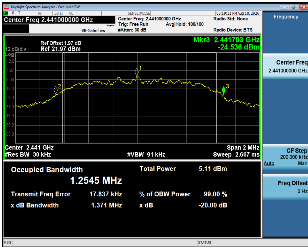
-20dB Bandwidth NVNT 2-DH5 2441MHz Ant1
