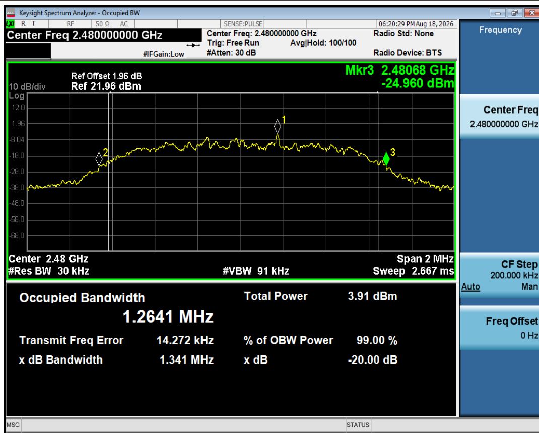
-20dB Bandwidth NVNT 2-DH5 2480MHz Ant1
