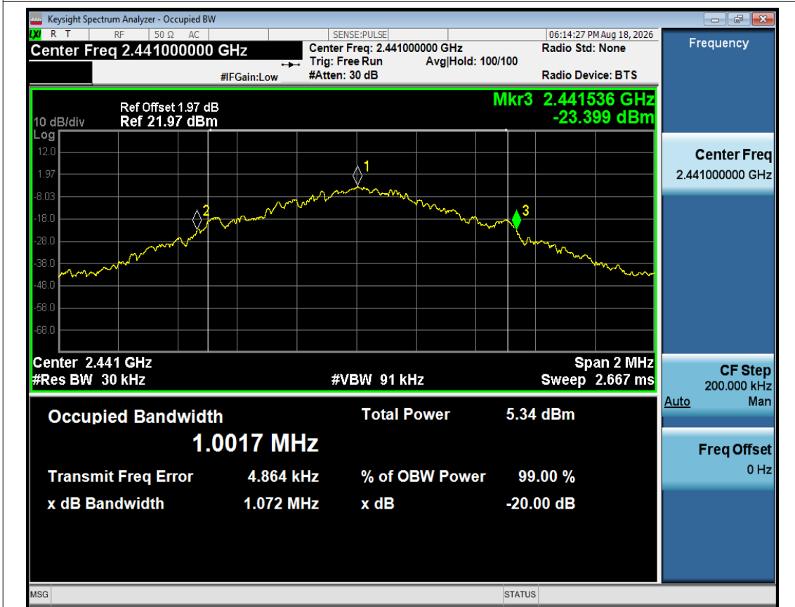
-20dB Bandwidth NVNT 1-DH5 2441MHz Ant1
