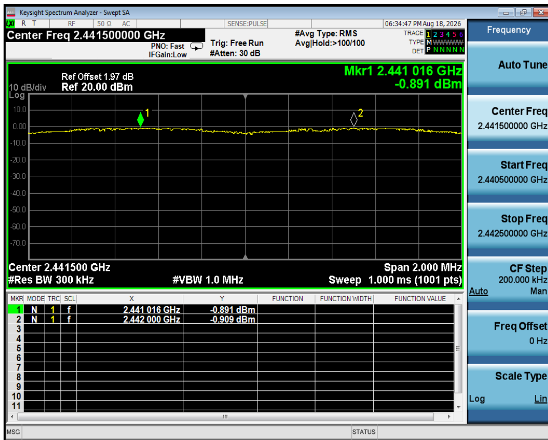
CFS NVNT 2-DH5 2441MHz Ant1
