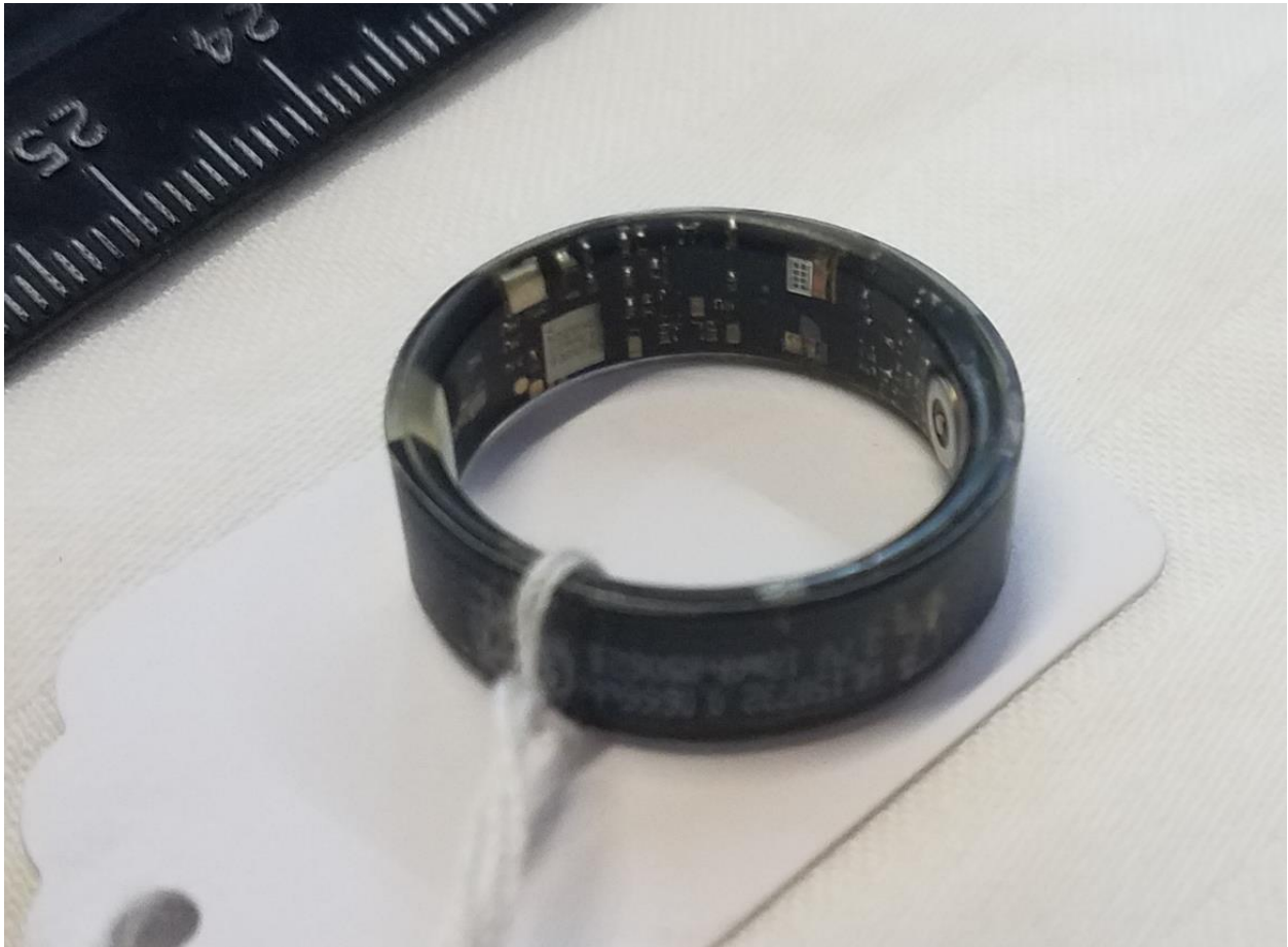
Figure 5. Main PCB in Ring (covered in clear epoxy)
