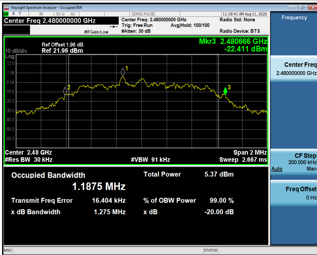
-20dB Bandwidth NVNT 2-DH1 2480MHz Ant1
