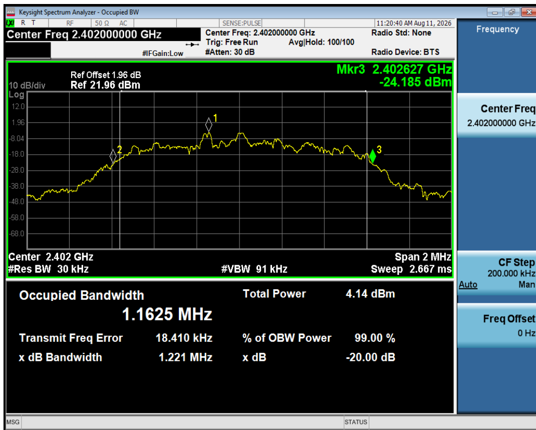
-20dB Bandwidth NVNT 3-DH1 2402MHz Ant1
