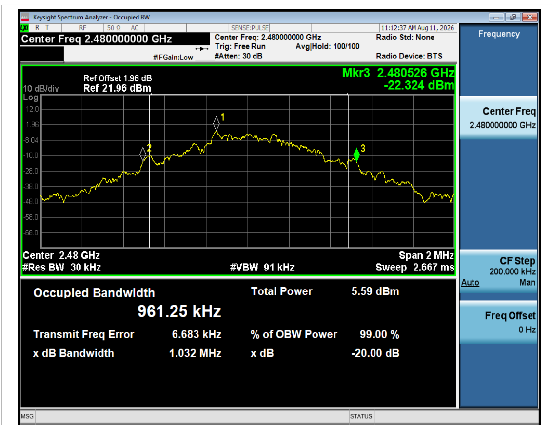
-20dB Bandwidth NVNT 1-DH1 2480MHz Ant1
