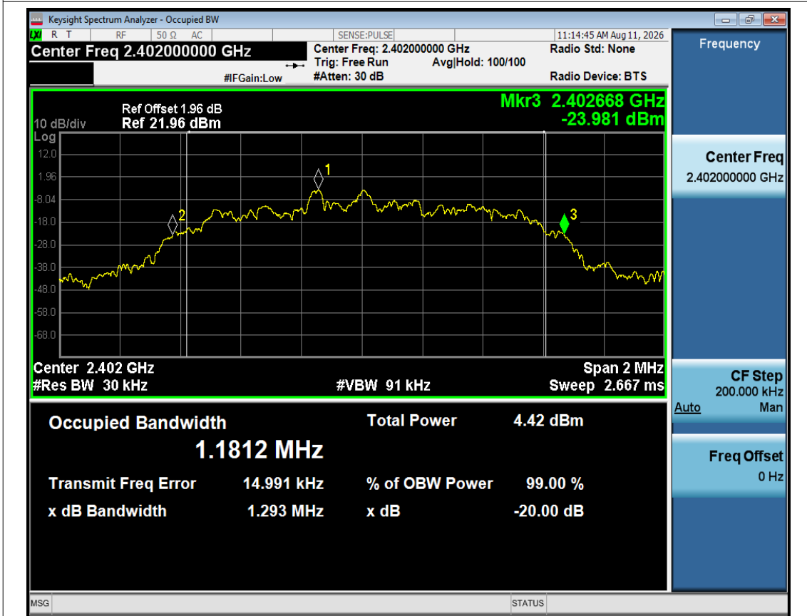
-20dB Bandwidth NVNT 2-DH1 2402MHz Ant1
