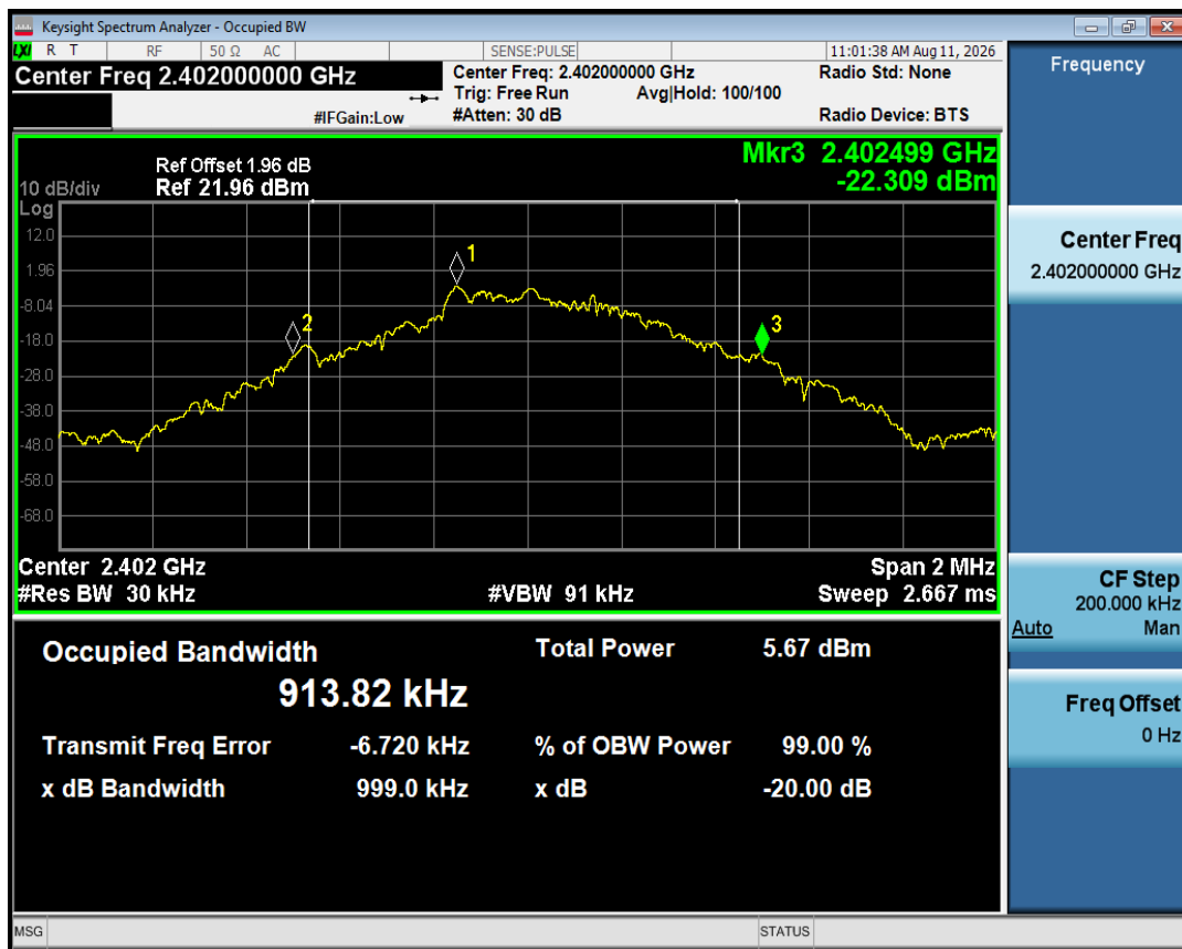
-20dB Bandwidth NVNT 1-DH1 2402MHz Ant1
