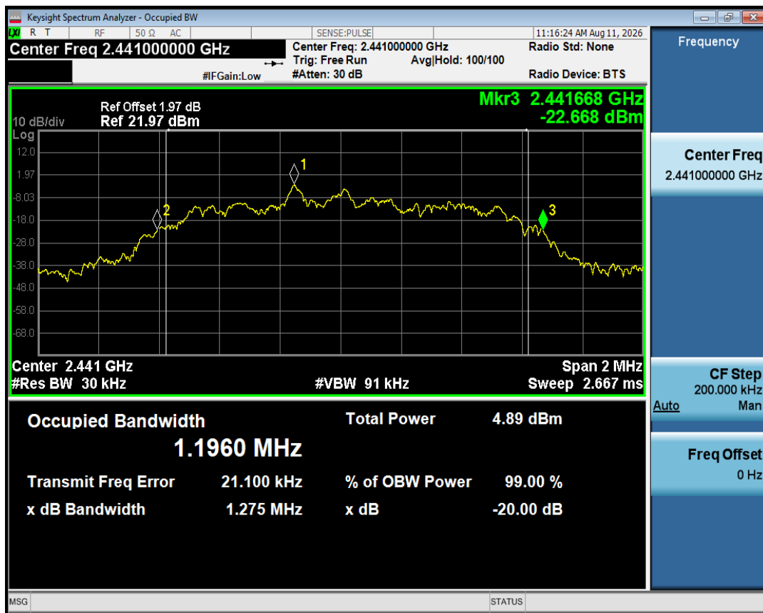
-20dB Bandwidth NVNT 2-DH1 2441MHz Ant1
