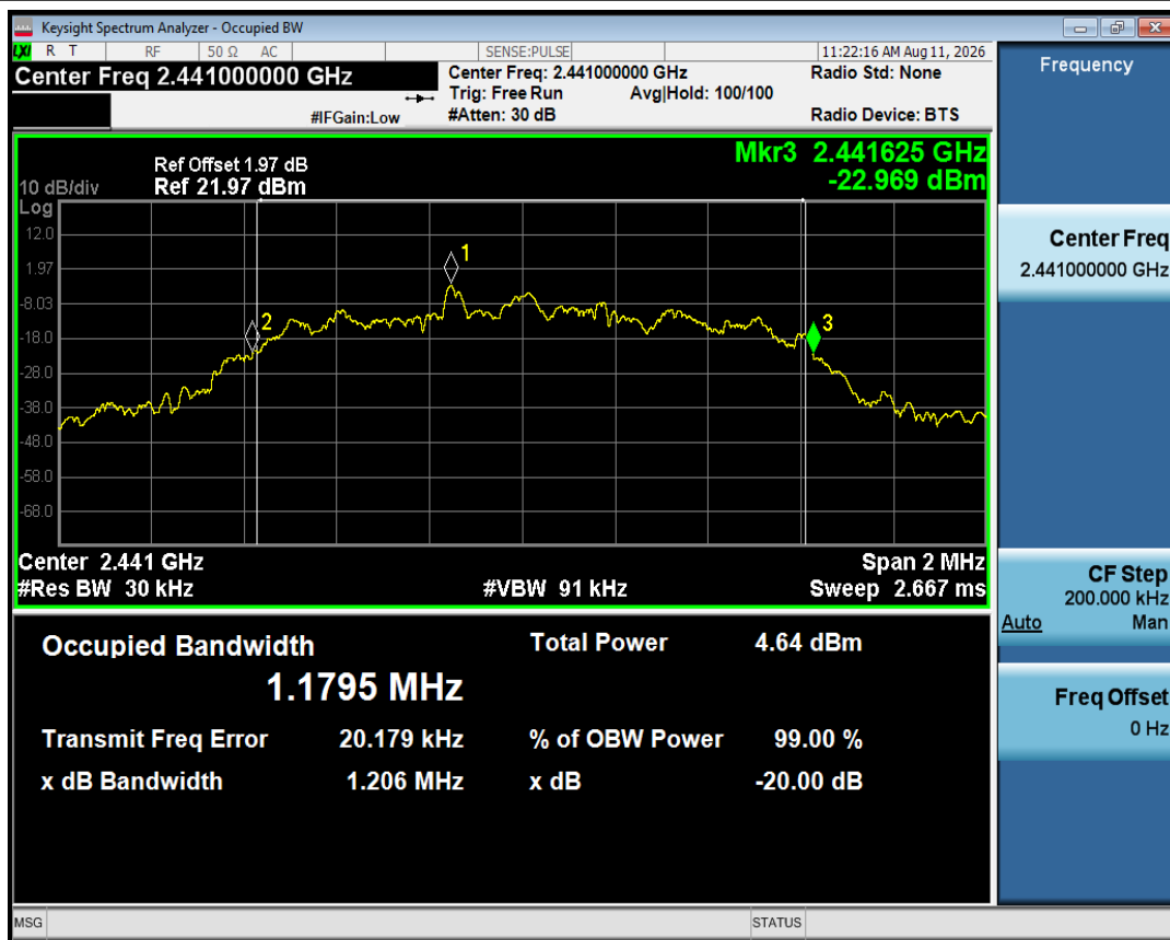
-20dB Bandwidth NVNT 3-DH1 2441MHz Ant1
