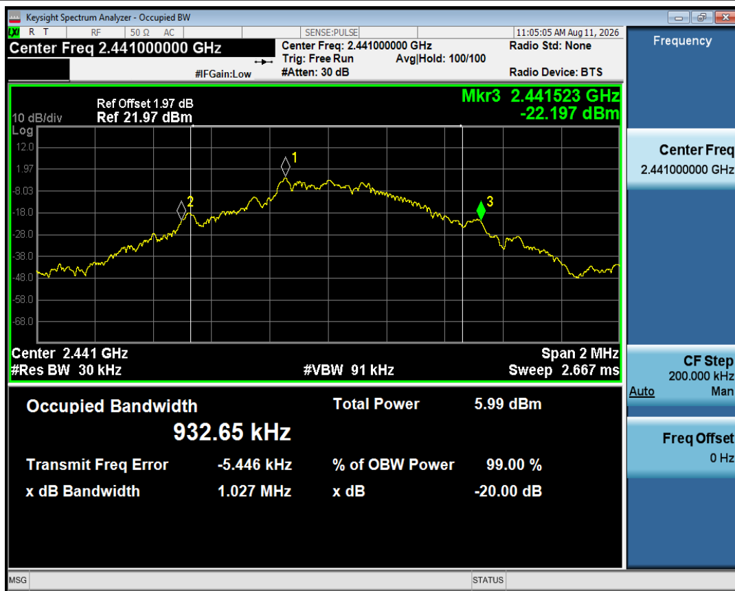
-20dB Bandwidth NVNT 1-DH1 2441MHz Ant1
