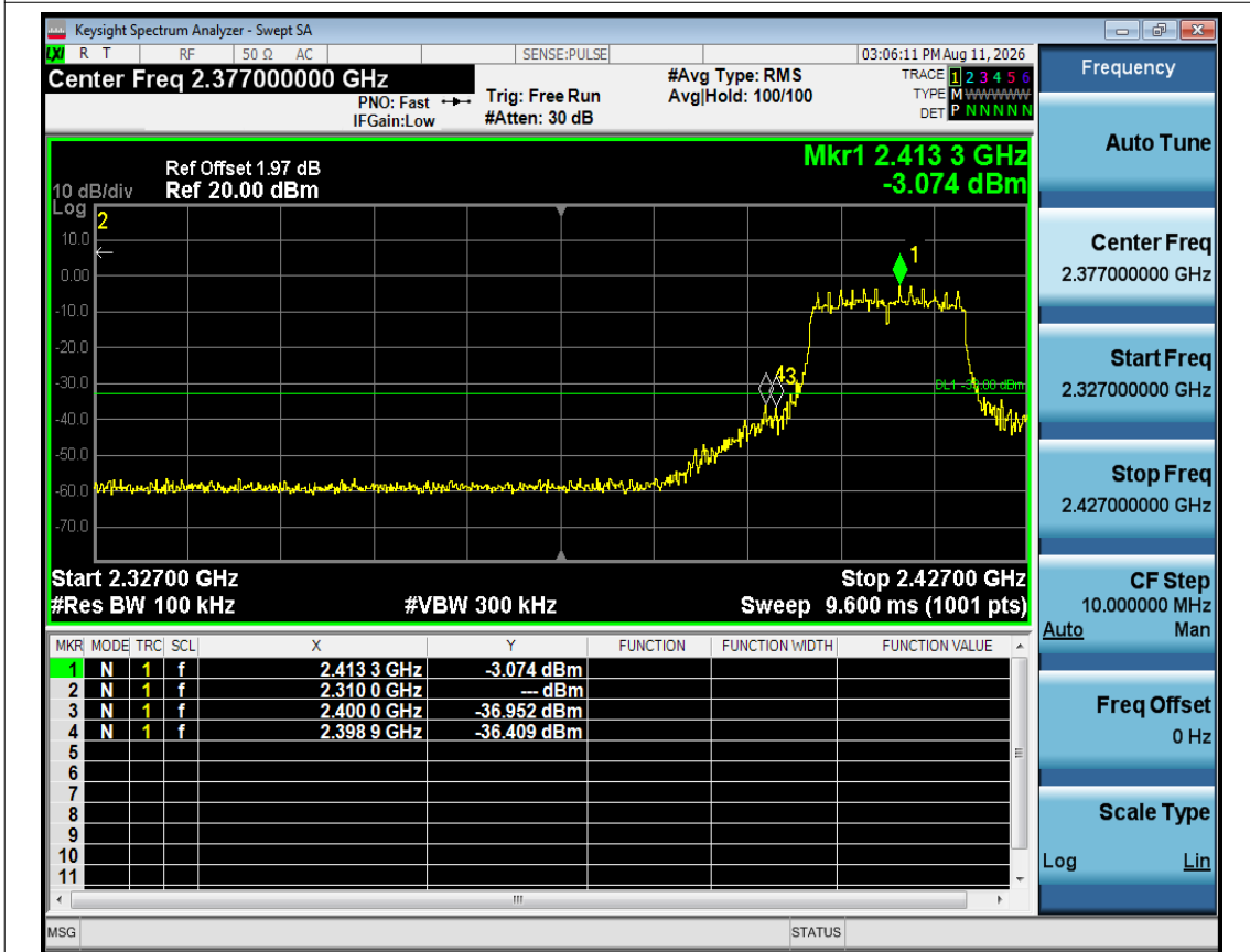
Band Edge NVNT g 2412MHz Ant1 Emission
