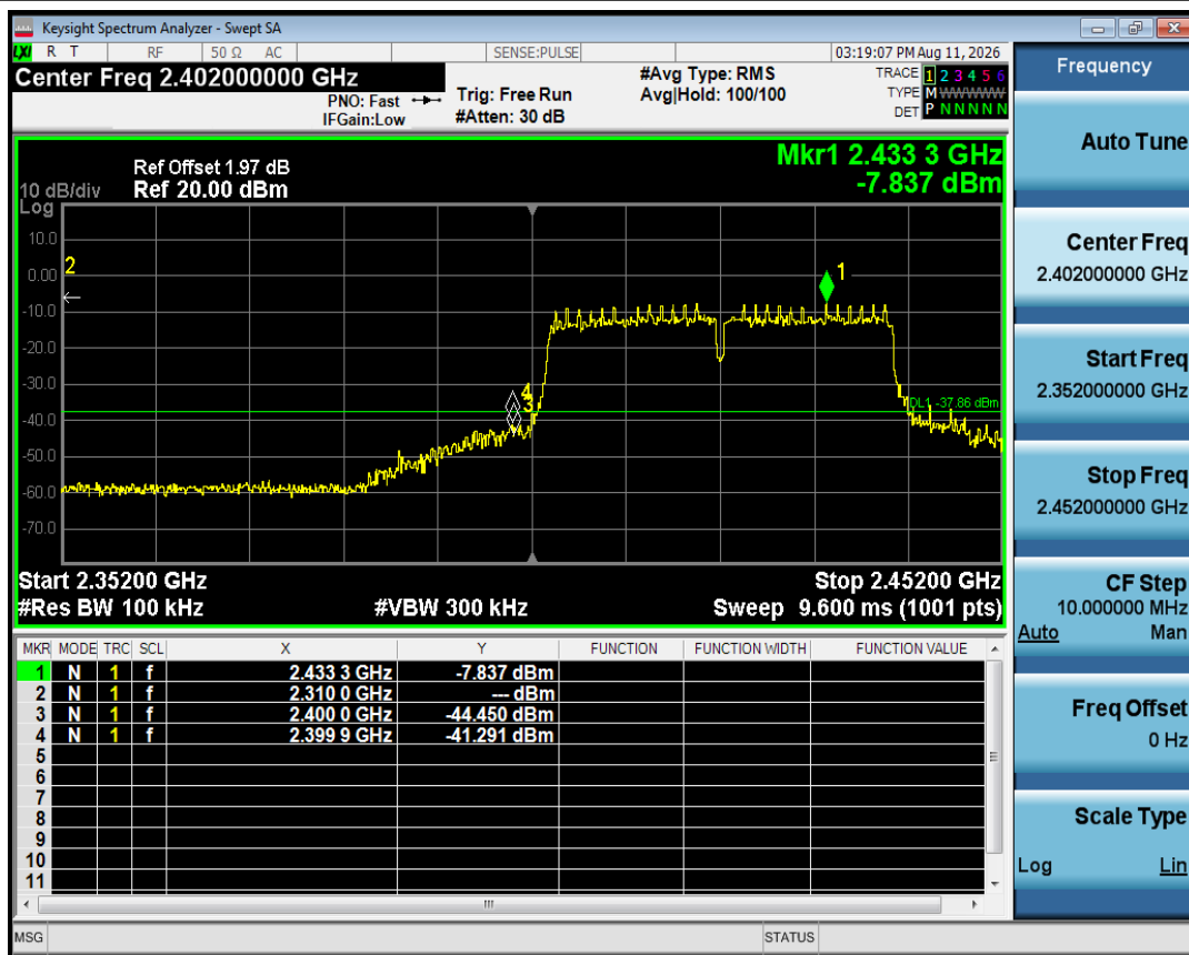
Band Edge NVNT n40 2422MHz Ant1 Emission
