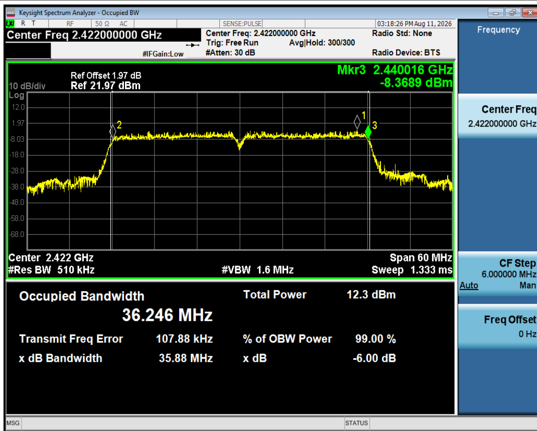
-6dB Bandwidth NVNT n40 2422MHz Ant1
