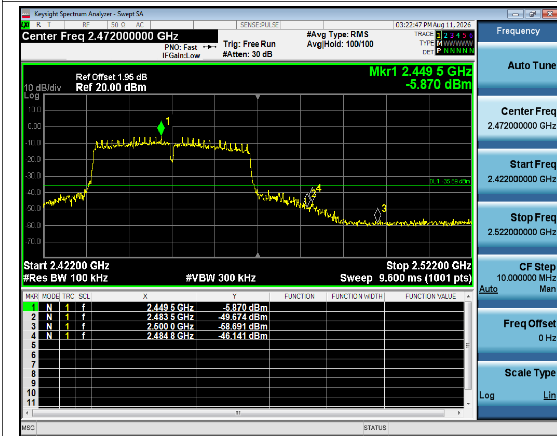
Band Edge NVNT n40 2452MHz Ant1 Emission
