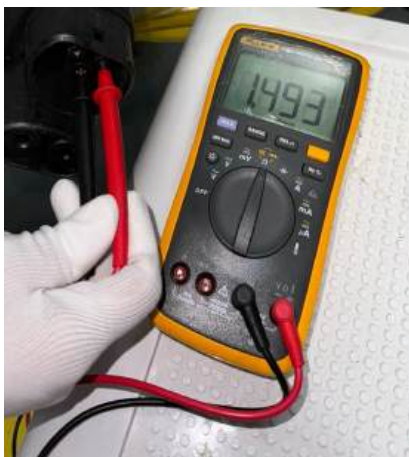
Figure 8-16 Measure the voltage between PE and PP
