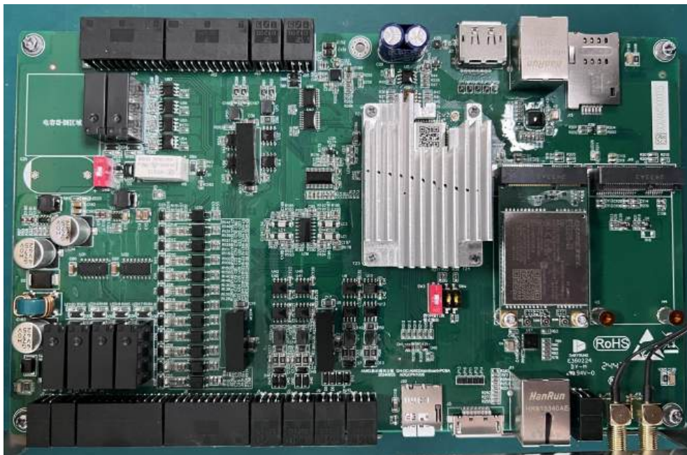
Figure 8-1 The AM62 core board and the AM62 board
