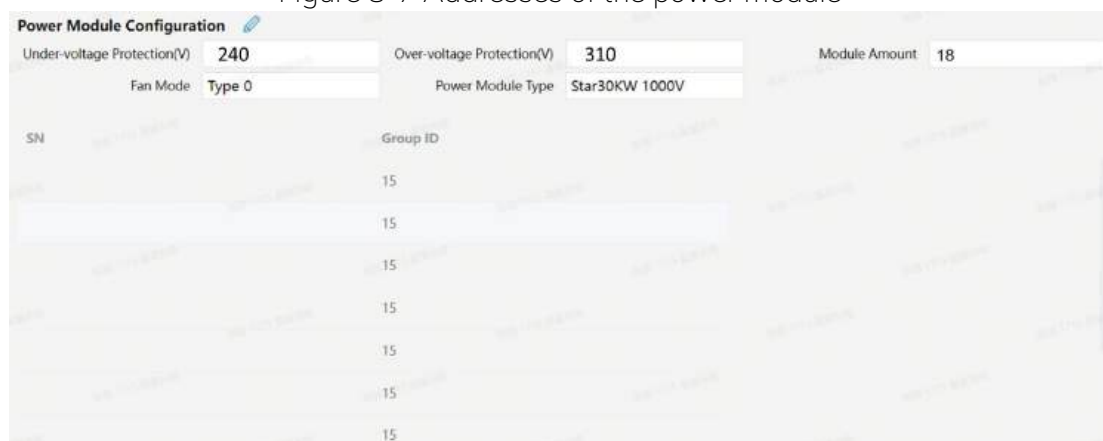
Figure 8-8 Configure the power modules in the web panel
