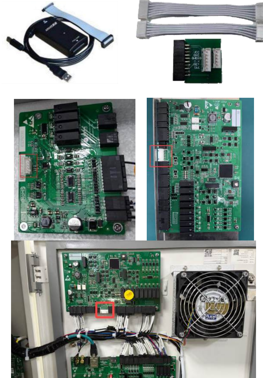
Figure 6-42 Update M4 board (CB02)/PDU control board/environmental monitoring board via Jlink #1
