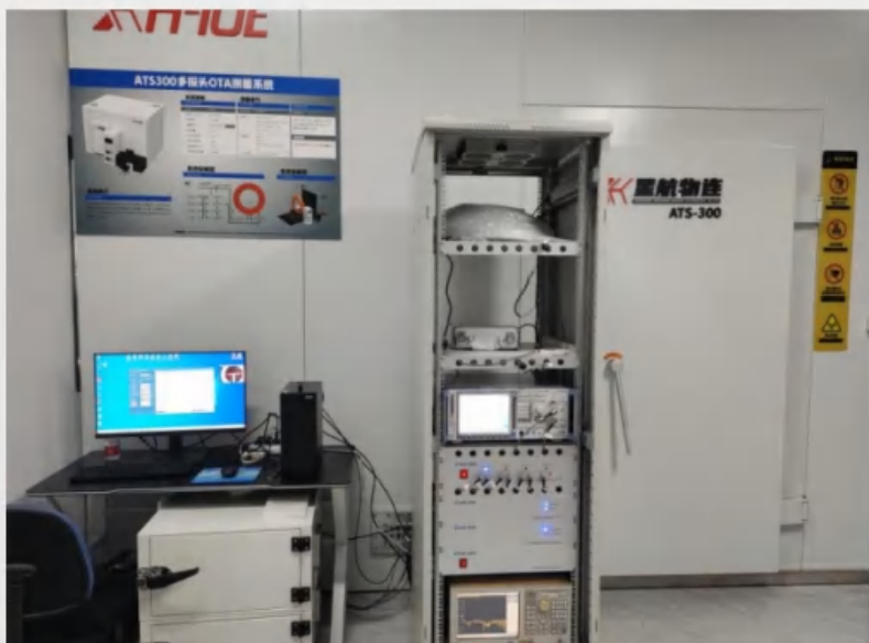
Figure 1. Test equipment and the fully anechoic chamber used for antenna characterization.
