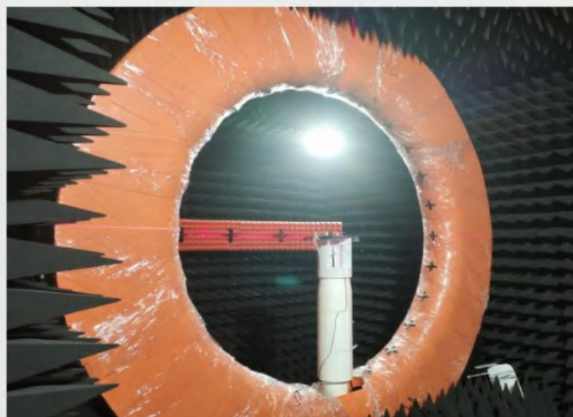
Figure 1. Test equipment and the fully anechoic chamber used for antenna characterization.
