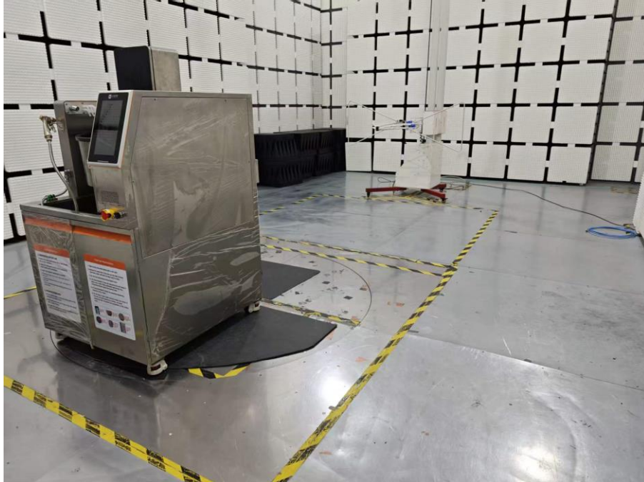
Set-up for Radiated Spurious Emission, Above 1GHz
