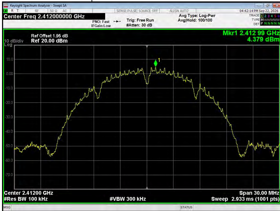
Tx. Spurious NVNT b 2412MHz Ant1 Emission
