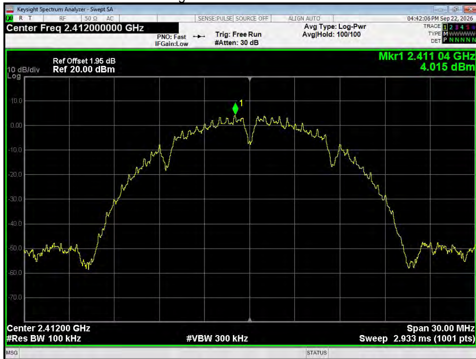
Band Edge NVNT b 2412MHz Ant1 Emission
