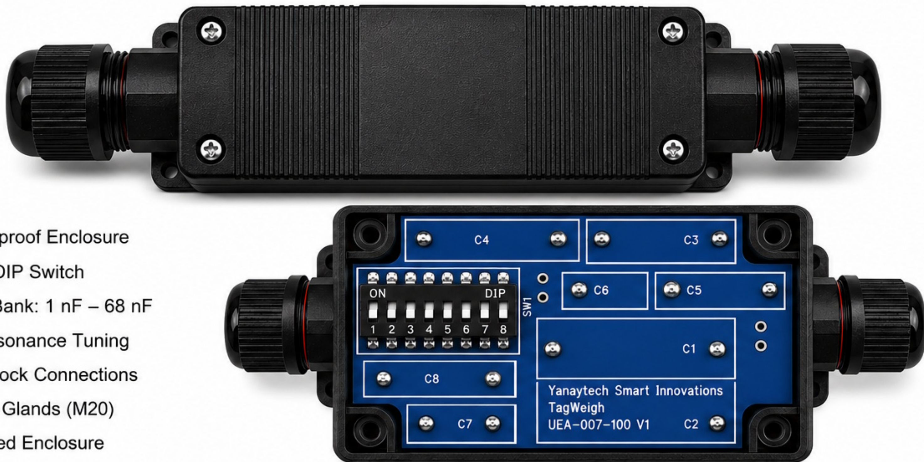
Inside view (DIP switch and capacitor bank)
