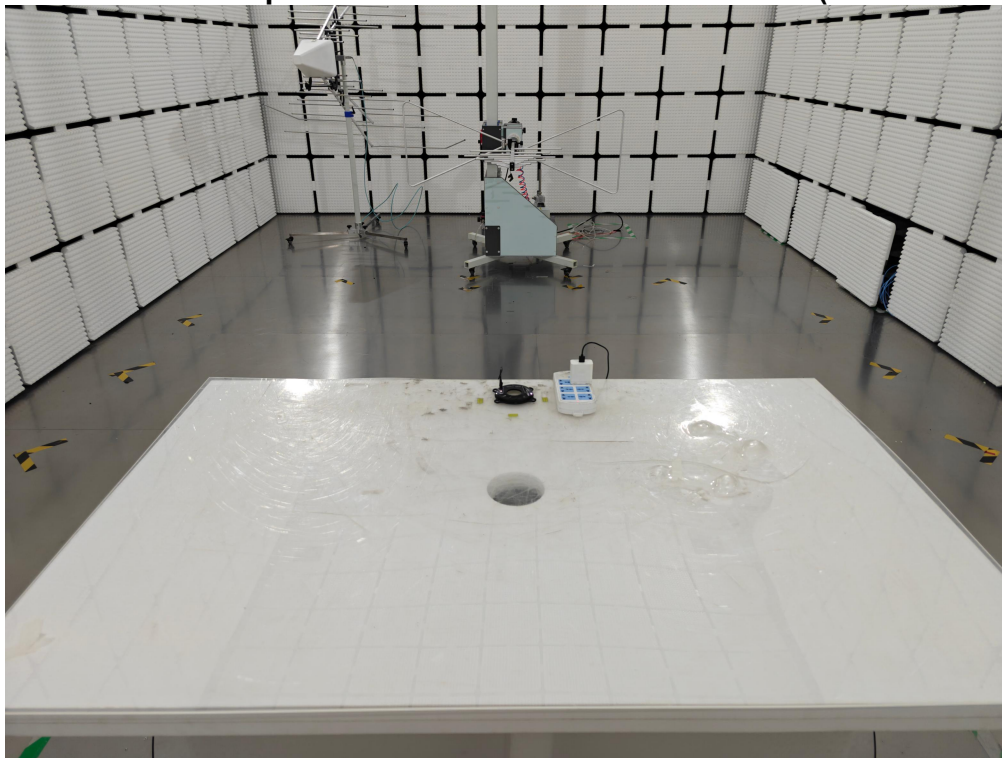
Photo 1 Test Setup Photos of Radiated Emission Test (30-1000MHz)
