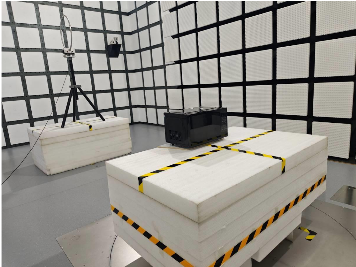
Radiated Emission 9 kHz-30 MHz Perpendicular Rear View
