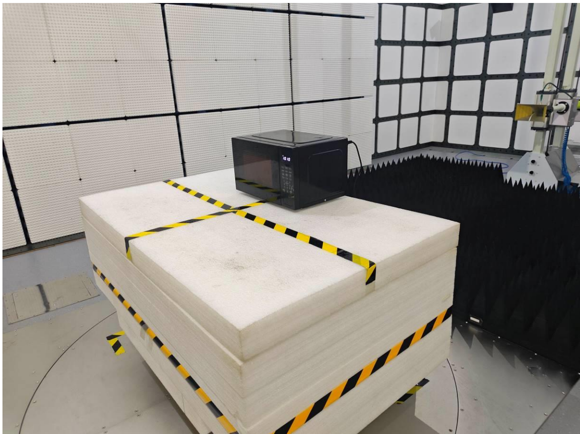
Radiated Emission Above 1GHz Rear View
