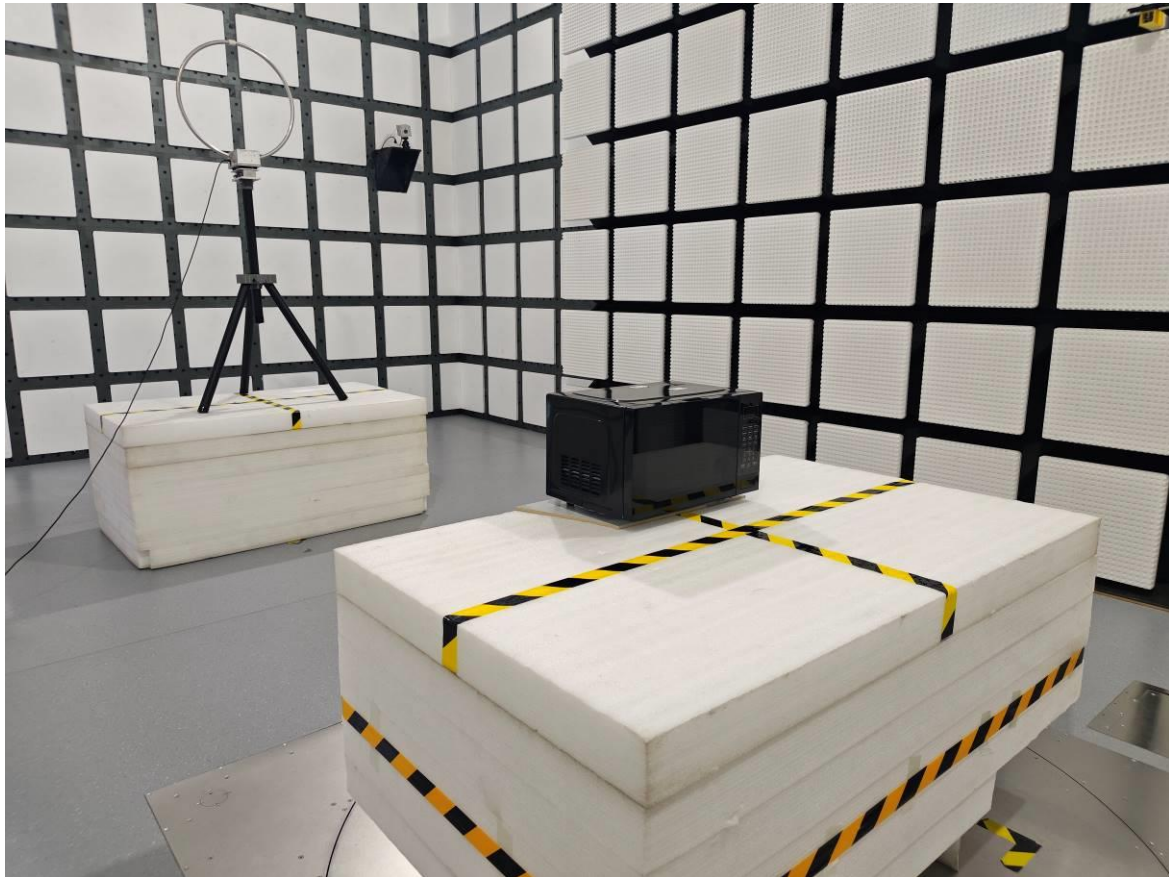
Radiated Emission 9 kHz-30 MHz Parallel Rear View
