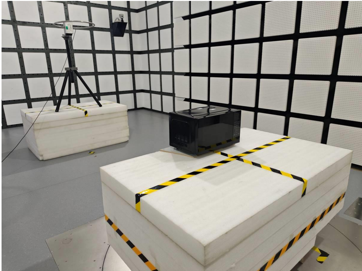
Radiated Emission 9 kHz-30 MHz Ground-parallel Rear View
