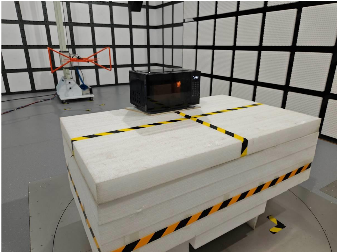
Radiated Emission 30 MHz-1 GHz Rear View
