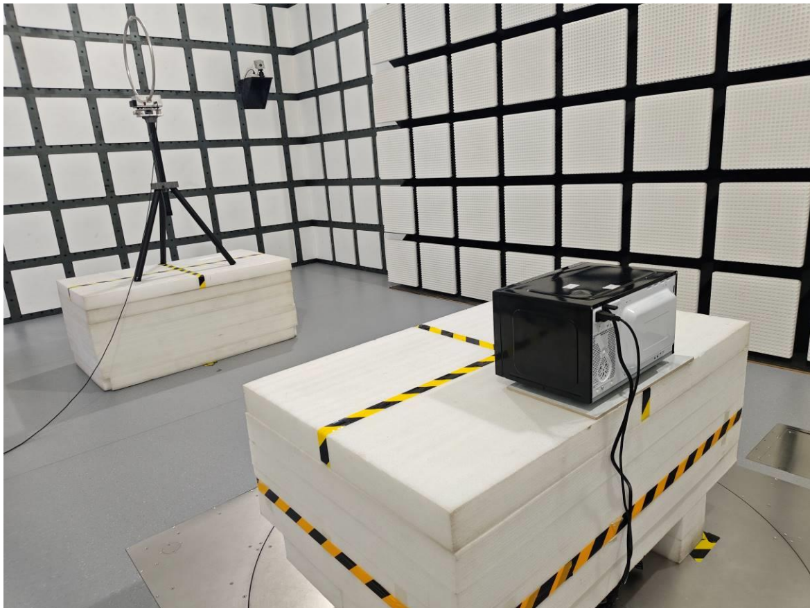
Radiated Emission 9 kHz-30 MHz Perpendicular Rear View
