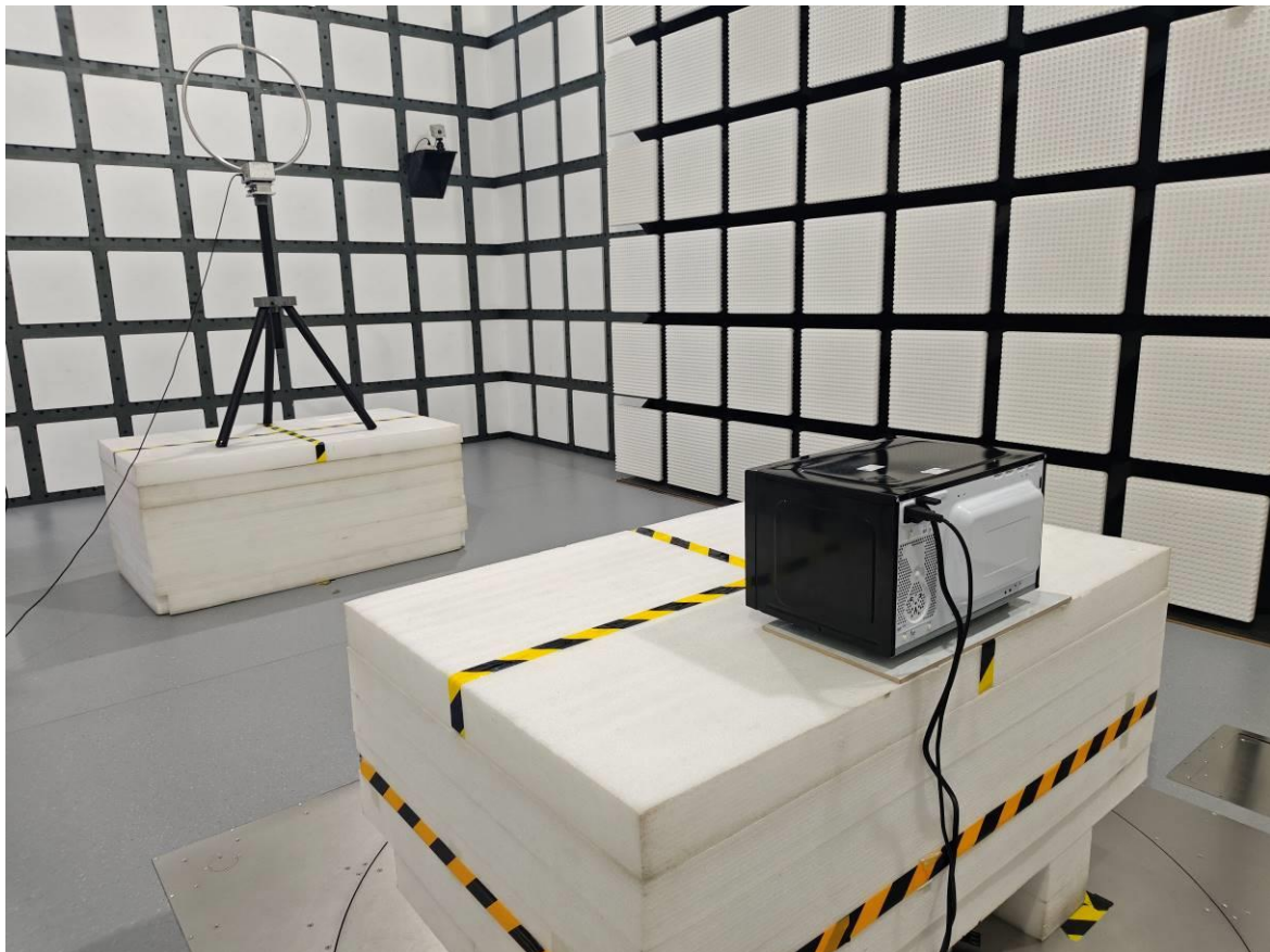
Radiated Emission 9 kHz-30 MHz Parallel Rear View
