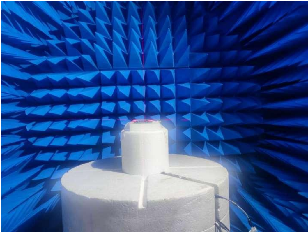
Figure 1. Test setup inside the anechoic chamber (coordinate fixture X/Y/Z).
