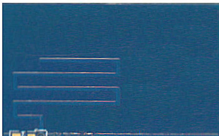
Figure 4. Part of 802.15.4 and BLE PCB with meander-like antenna (scale approximately 4:1)
