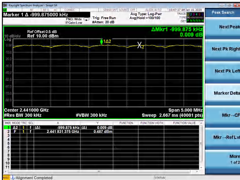
Figure 26: Frequency Separation, TM18, observation Frequency 2441MHz
