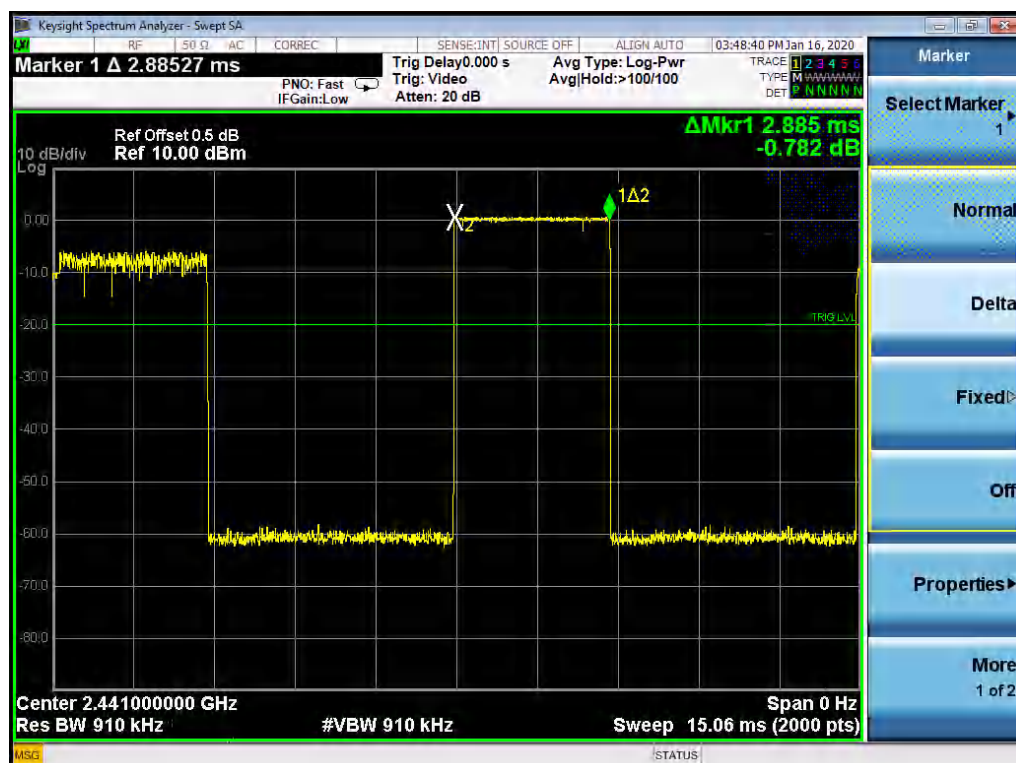
Figure 45: Time of Occupancy, TM15, observation Frequency 2441MHz
