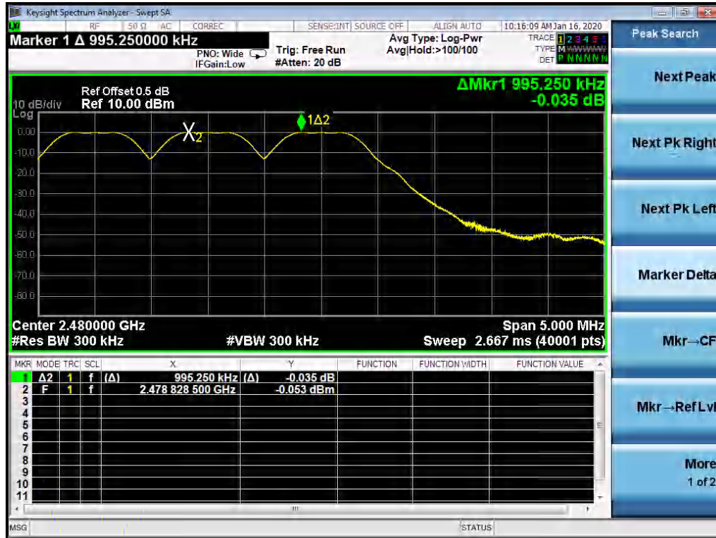
Figure 21: Frequency Separation, TM12, observation Frequency 2480MHz
