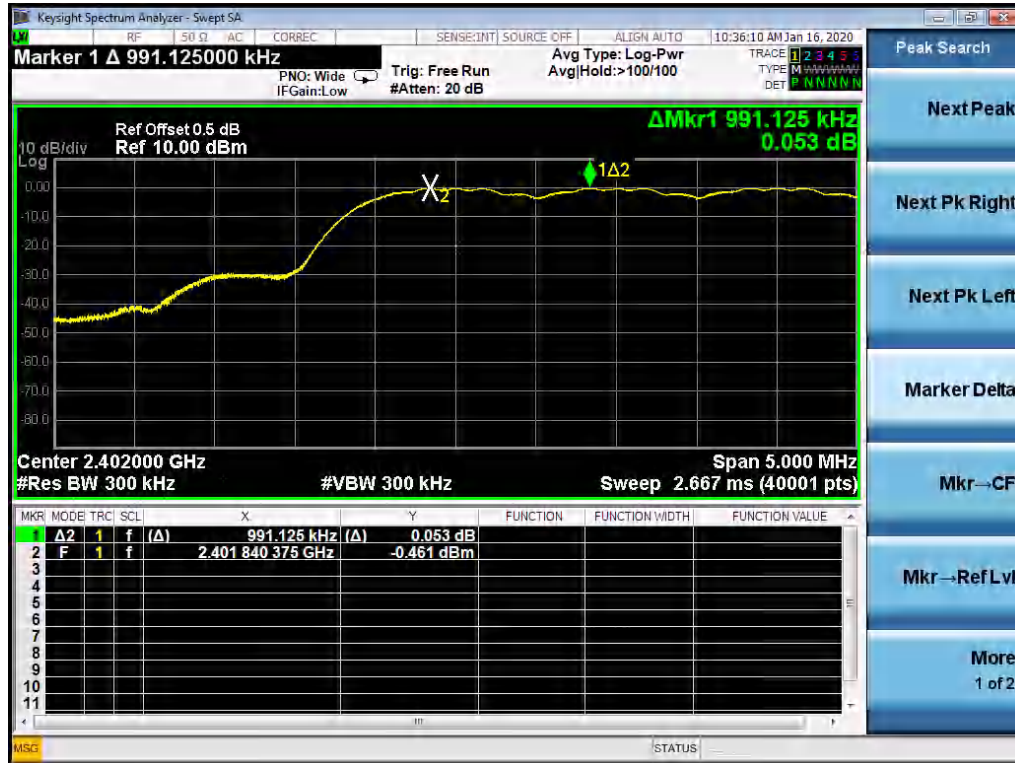
Figure 25: Frequency Separation, TM18, observation Frequency 2402MHz
