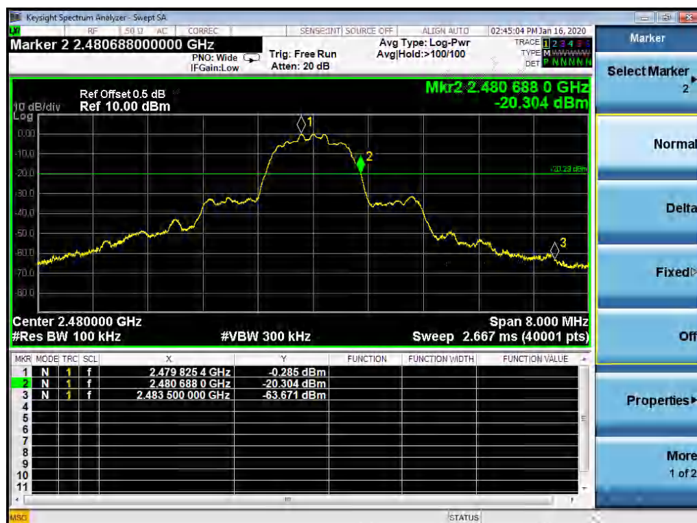
Figure 54: Conducted Band-Edge, TM9
