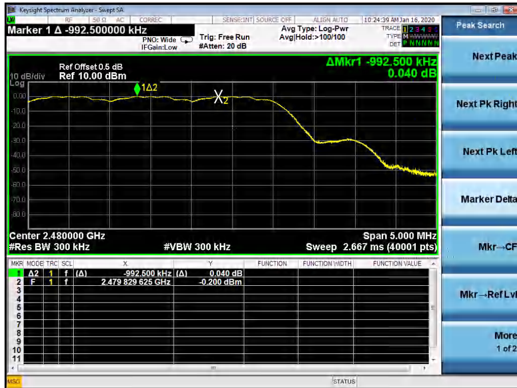
Figure 27: Frequency Separation, TM18, observation Frequency 2480MHz
