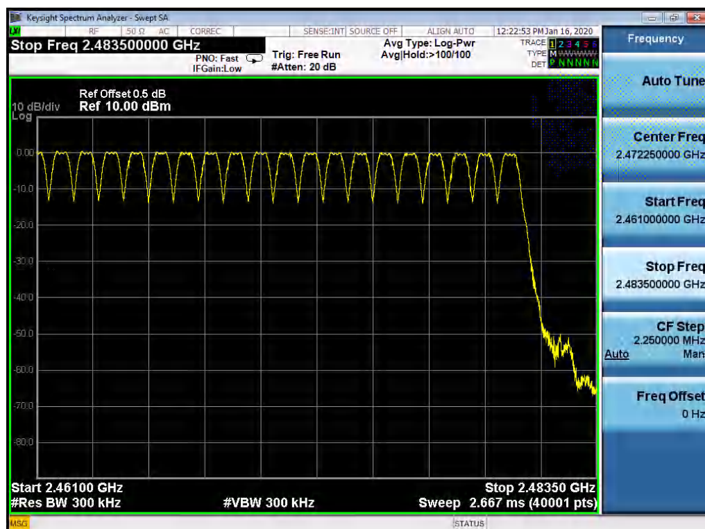
Figure 31: Number of Hopping Frequency, TM12, part 4
