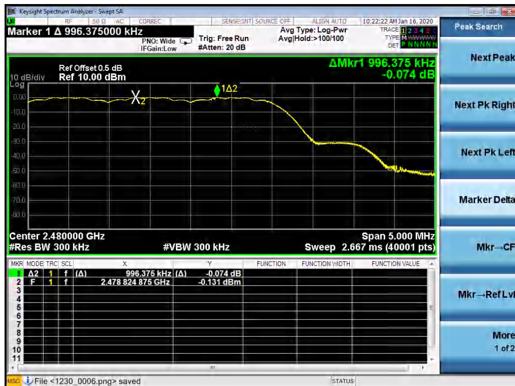
Figure 24: Frequency Separation, TM15, observation Frequency 2480MHz
