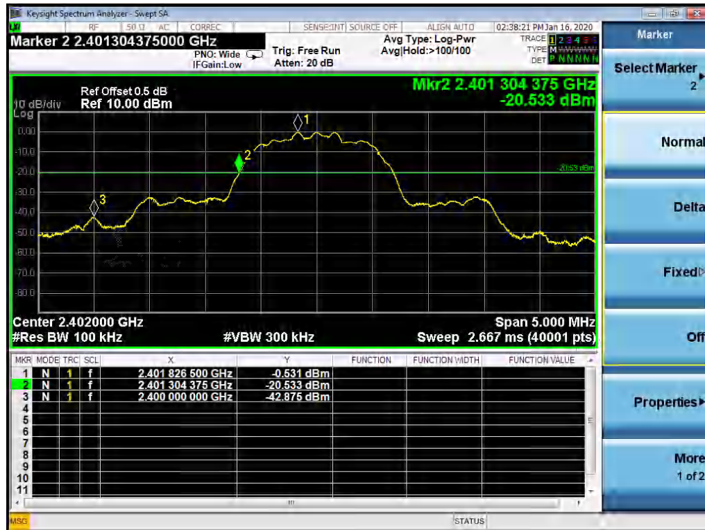
Figure 53: Conducted Band-Edge, TM7
