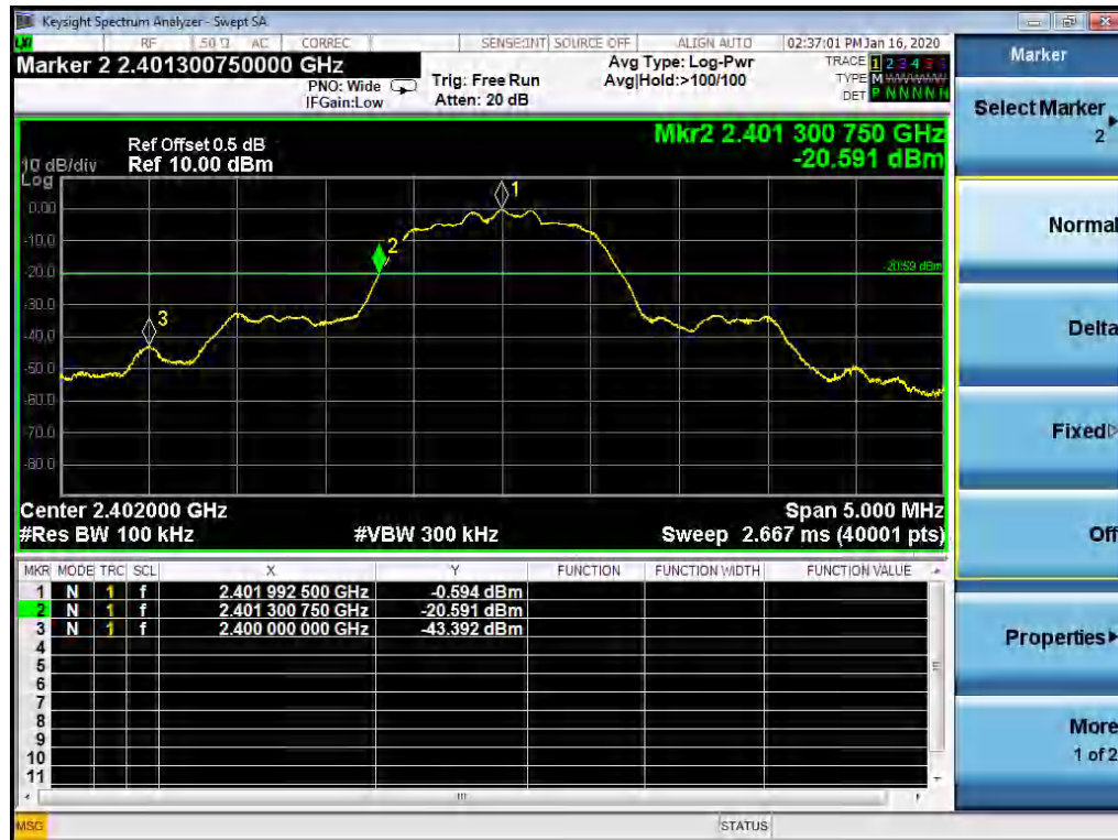
Figure 51: Conducted Band-Edge, TM4
