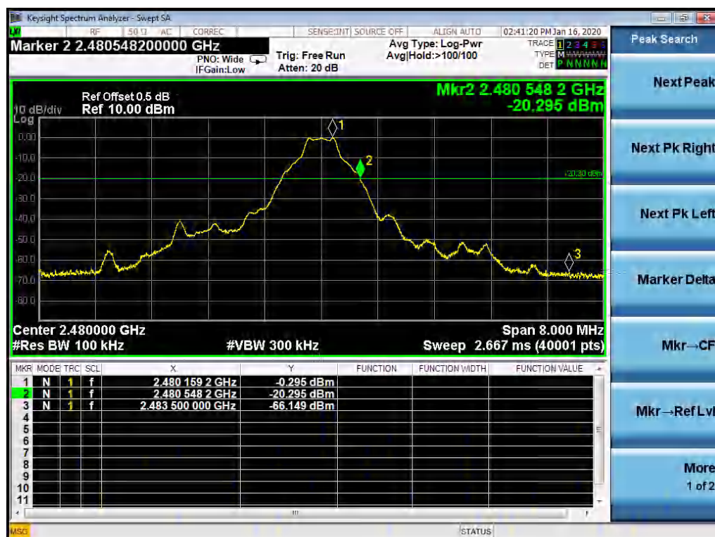
Figure 50: Conducted Band-Edge, TM3
