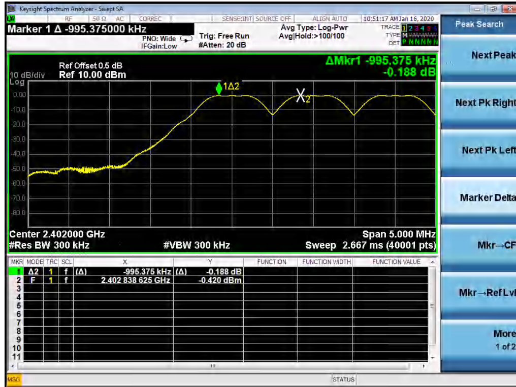
Figure 19: Frequency Separation, TM12, observation Frequency 2402MHz
