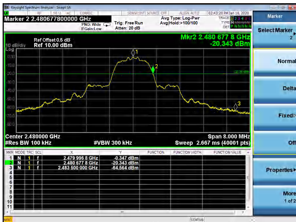
Figure 52: Conducted Band-Edge, TM6
