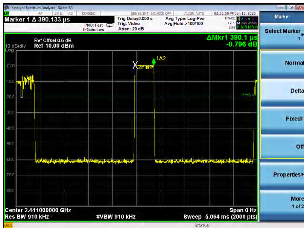
Figure 43: Time of Occupancy, TM13, observation Frequency 2441MHz
