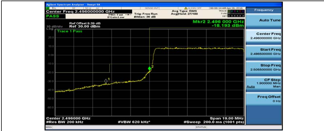
Channel Bandwidth: 10 MHz_HCH_16QAM_1RB#0
