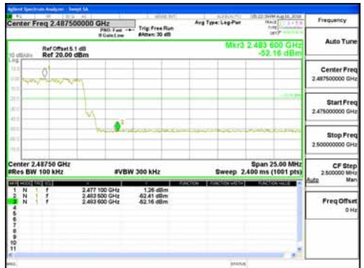
Hopping Band Edge_8DPSK_3M_DH5_2480MHz
