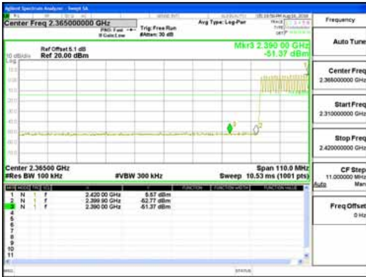
Hopping Band Edge_GFSK_1M_DH5_2480MHz
