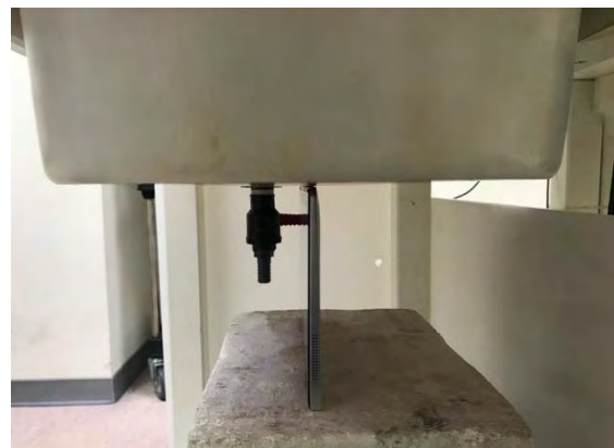
Fig.4 EUT Top side to flat phantom
