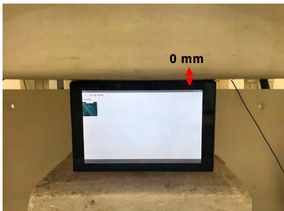
Fig.4 EUT Top side to flat phantom
