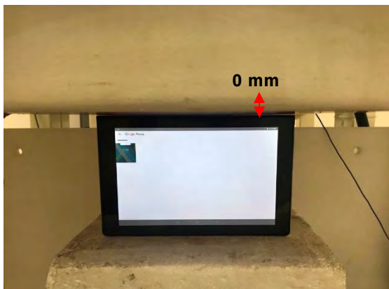
Fig.7 EUT Bottom side to flat phantom
