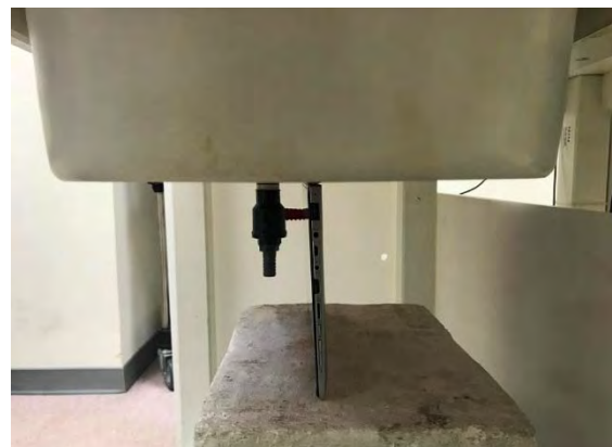
Fig.7 EUT Bottom side to flat phantom
