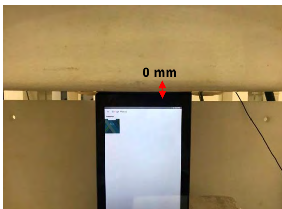
Fig.5 EUT Right side to flat phantom
