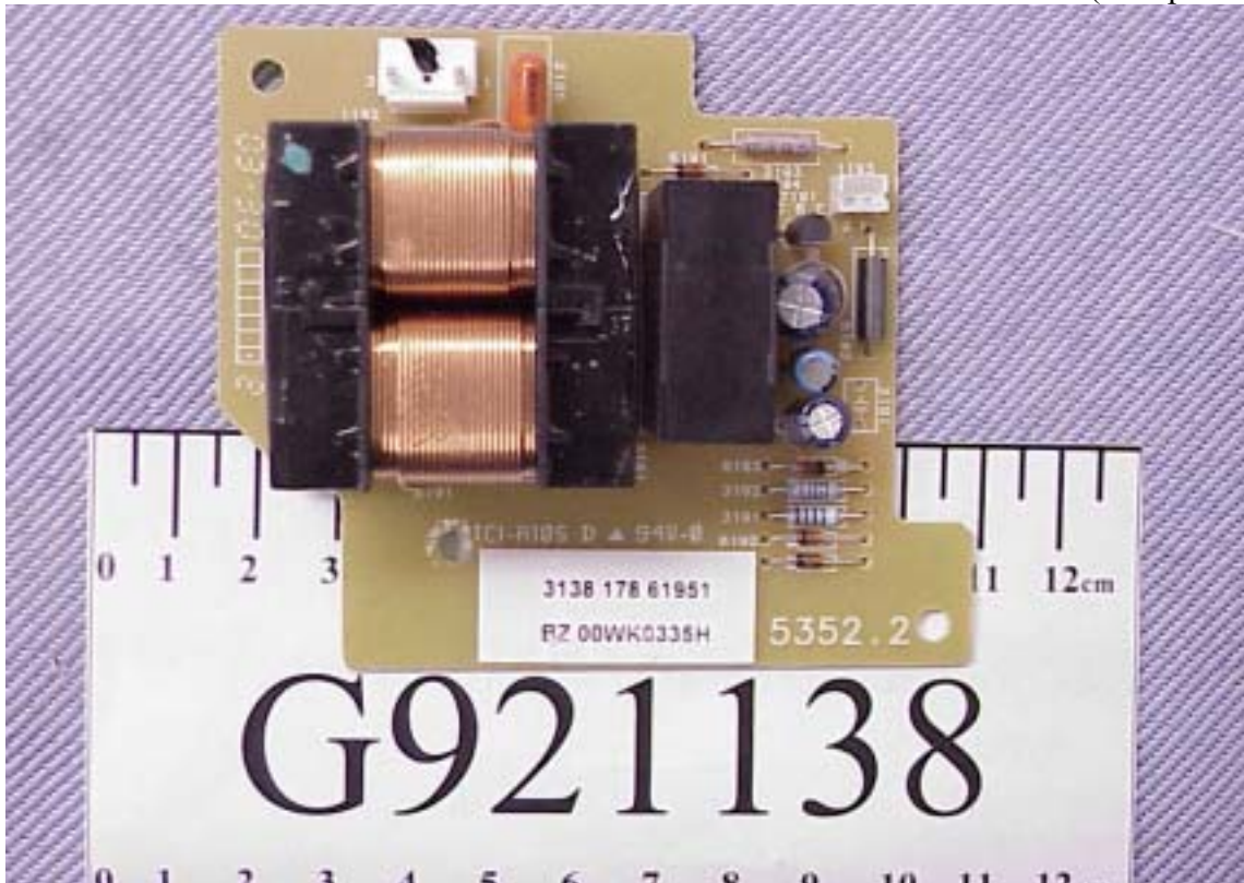
Figure 20 Display Color Monitor Transformer Board (Component View)
