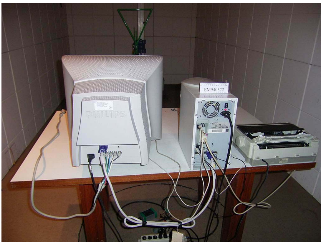
BACK VIEW OF RADIATED MEASUREMENT
