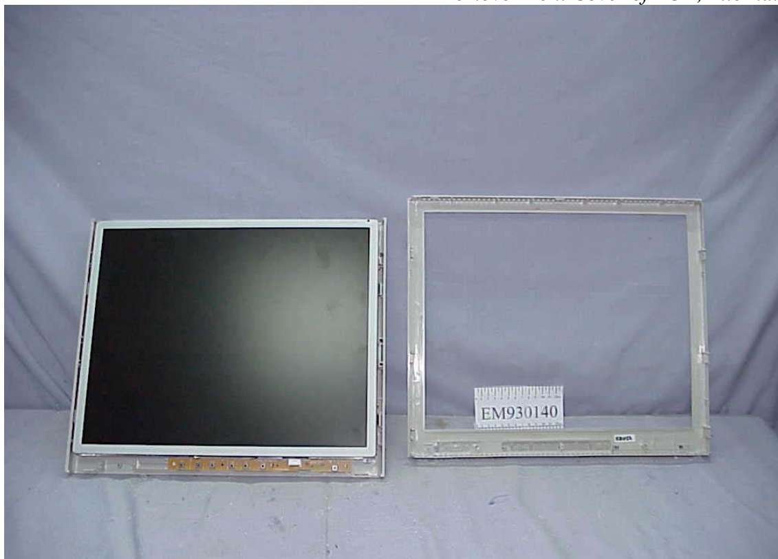
Figure 5 Remove Front Cover of LCD, Internal View
