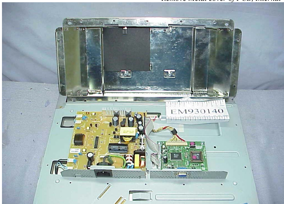
Figure 10 Remove Metal cover of PCB, Internal View
