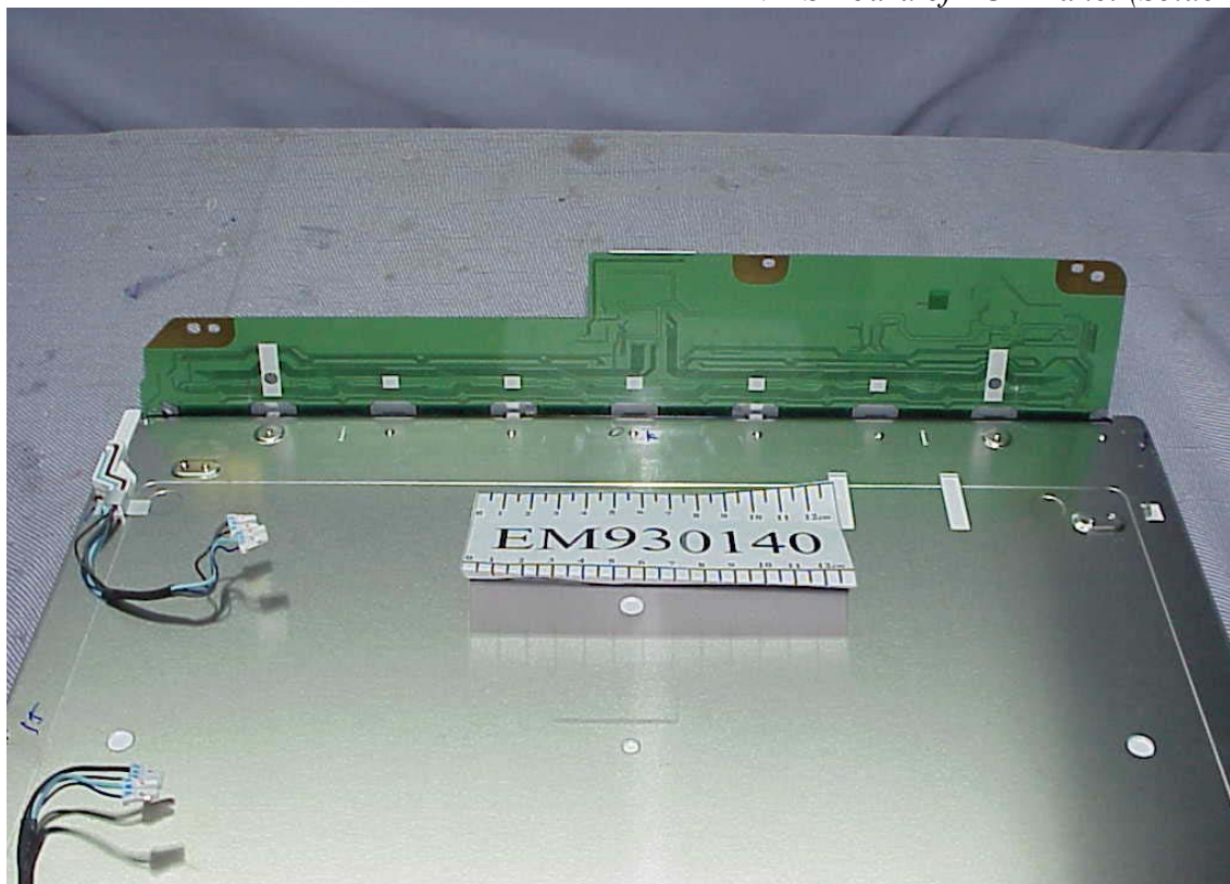
Figure 21 LVDS Board of LCD Panel (Solder Side)
