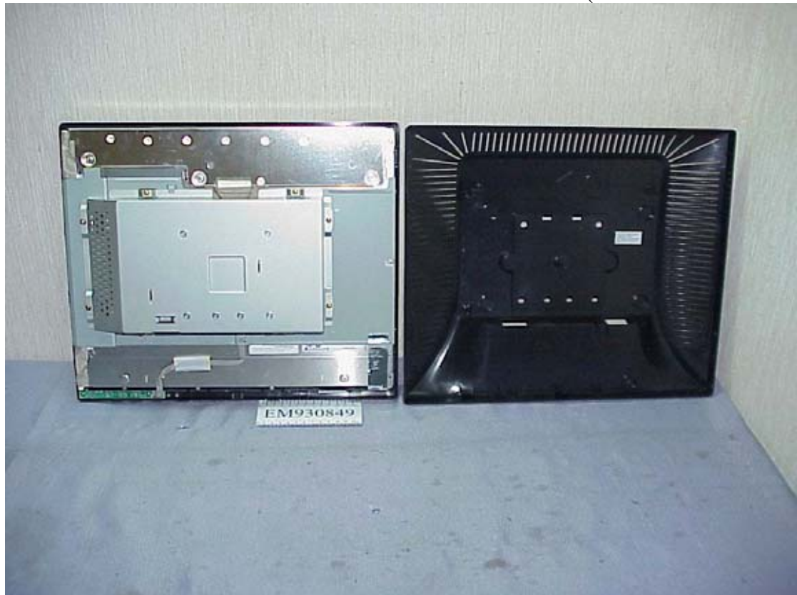
Figure 7 Internal View (Removed Back Cover)
