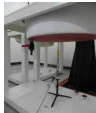
Photo of the dipole Antenna
