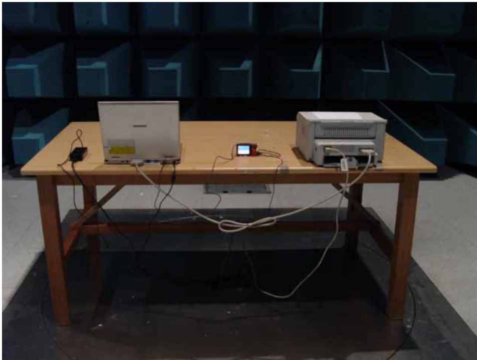
Picture 4. Radiated Emission (Rear)
