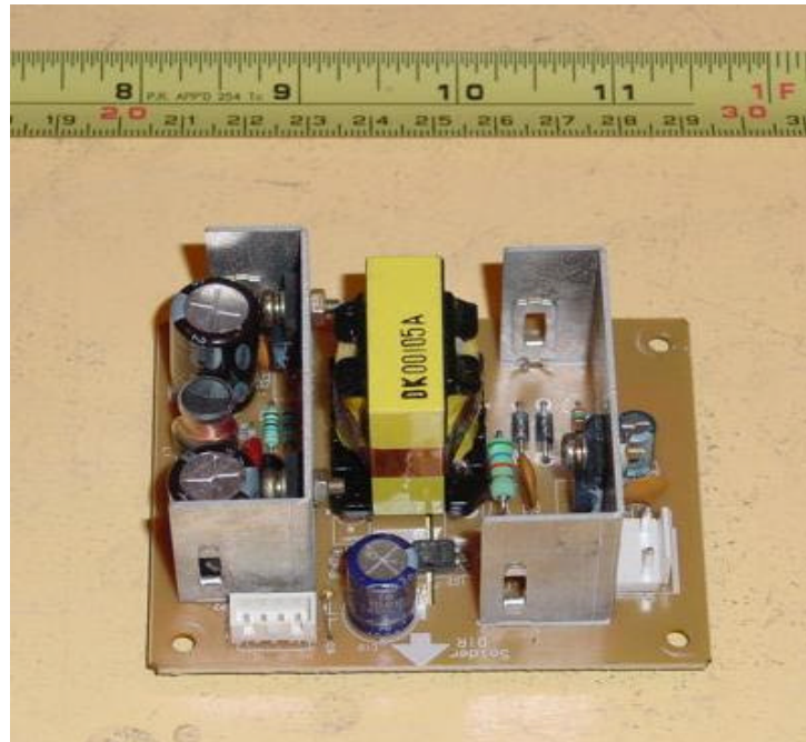
Front of Sub Power Board
