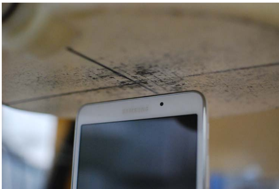
SAR Test Setup Photo 4 – Top Edge at 0.9 cm
