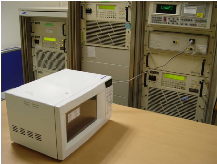
Fig.3 Test Setup for RF output power
