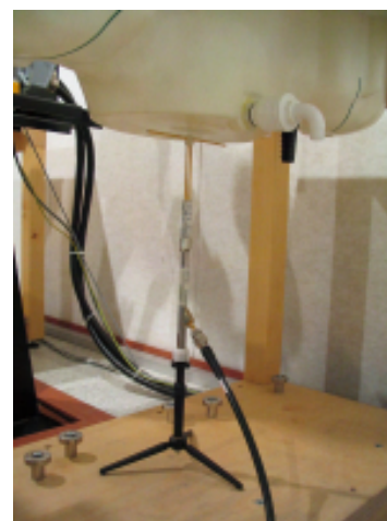
Photo of the dipole Antenna
