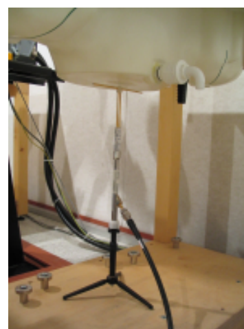
Photo of the dipole Antenna
